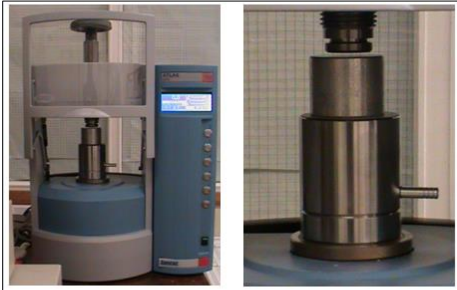
Figure 5-2 Specac Atlas T25 Automatic Hydraulic Press used to press membrane discs.
