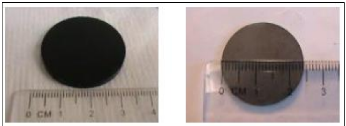
Figure 5-3 The 32mm Dia, 2mm thick pressed ceramic green body and the 25mm Dia, 1mm thick disc sintered at 1150°C.
