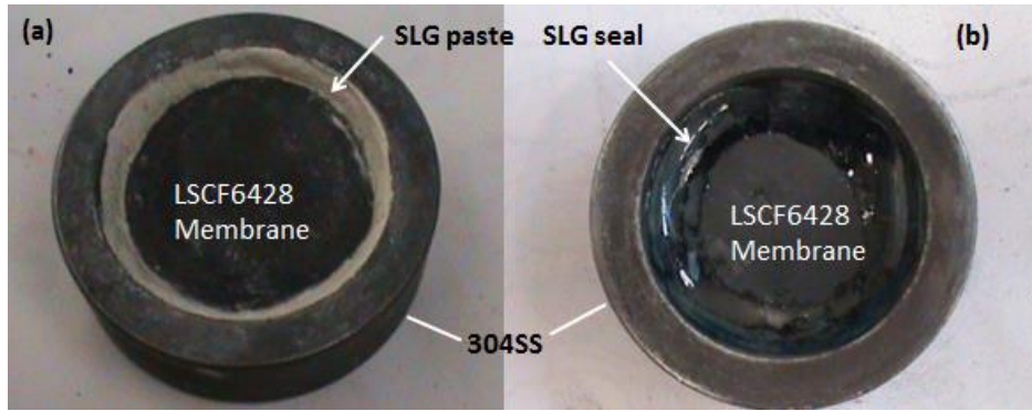
Figure 4-7 Images of membrane module: (a) assembly before sealing, (b) assembly after sealing
