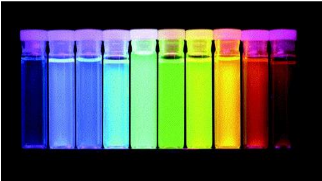
Figure 1. 2 The image shows ten luminescent colors of CdSe with ZnS shell QDs excited with a near-UV lamp. The colors show the range of particles sizes started from small to bigger size left to right (blue to red). The wavelengths correspond to fluorescent colors are 443, 473, 481, 500, 518, 543, 565, 587, 610, and 655 nm, respectively (Chan et al., 2002).
