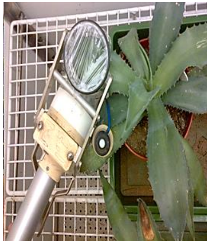
Figure 2.2 Leaf gas exchange measurements made by clamping cuvette on fully expanded Agave leaves.
