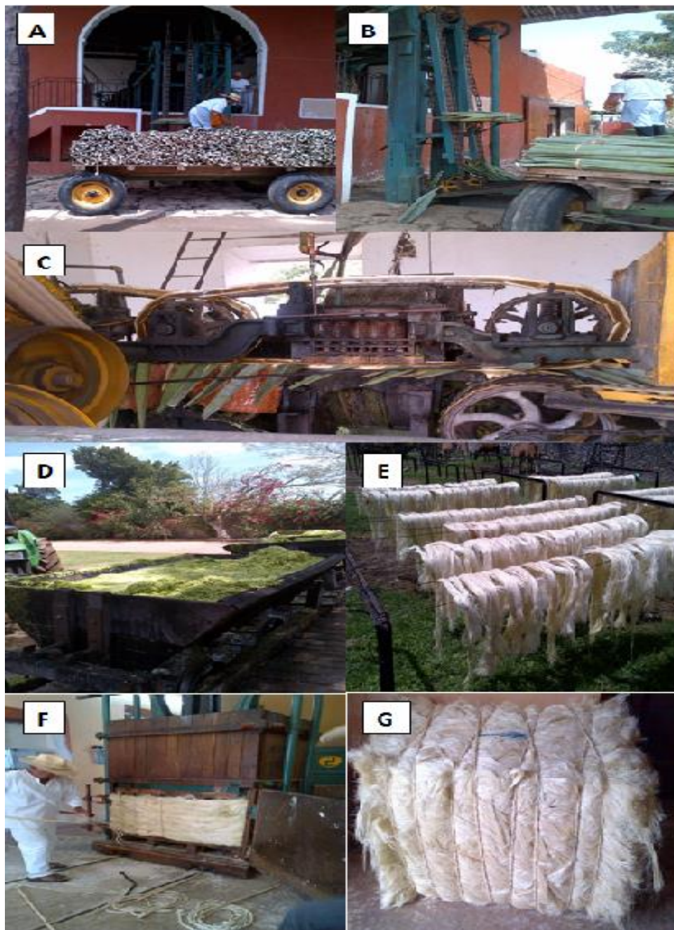
Figure 1.8 Process to obtain natural fibres from sisal. (A &B) Leaves of A. sisalana collected from the field. C) Decortication process. D) Juice extraction and bagasse used as fertilizer and animal feed. E) Drying of sisal fibres. F) Packing of natural sisal fibre. G) End product after compression of sisal. All photographs were taken in Sotuta De Peon Hacienda, Mexico, 2012.
