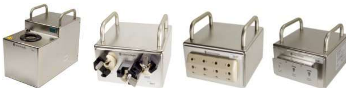
Image 10: Images of the modules used on the Modular Lab system. (left) Peltier reaction module (PRM) (left middle) Single stopcock modules (SSM) (right middle) Solenoid valve modules (SVM) (right) Vial holder module (VHM) 286
