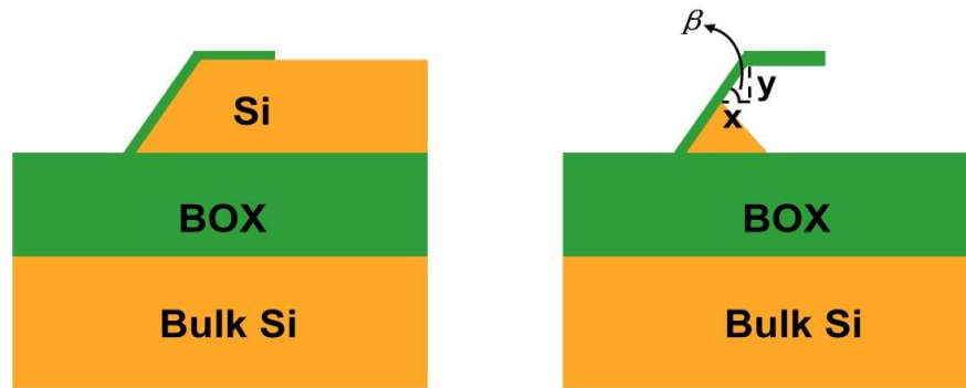
Figure 3.9: Schematic of the process steps involved during in situ size reduction of nanowires.
