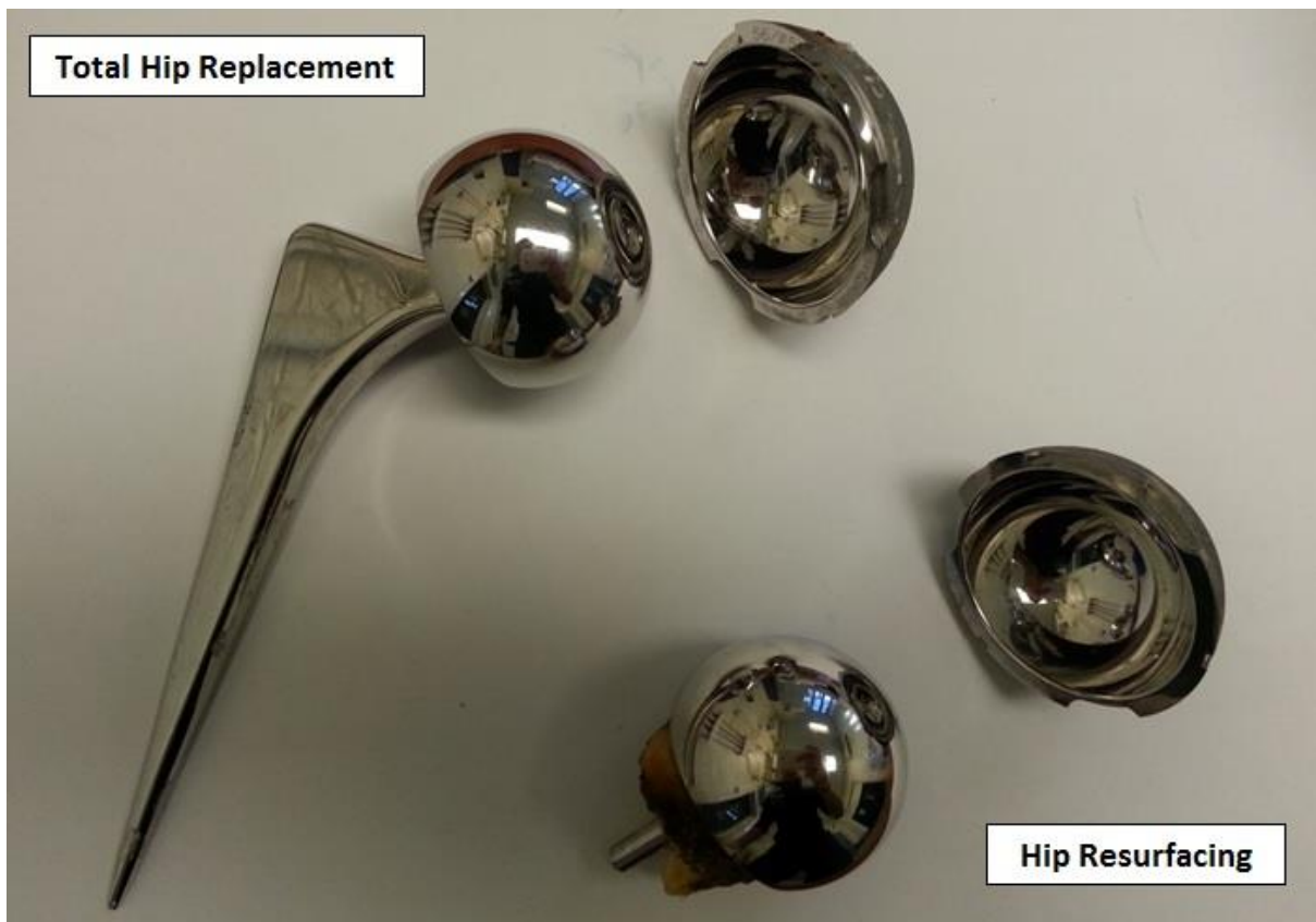
Figure 4: Photo of the Zimmer MoM Durom THR prosthesis (top left) and the Durom hip resurfacing prosthesis (bottom right). Note that both prostheses utilise the same design of acetabular component
