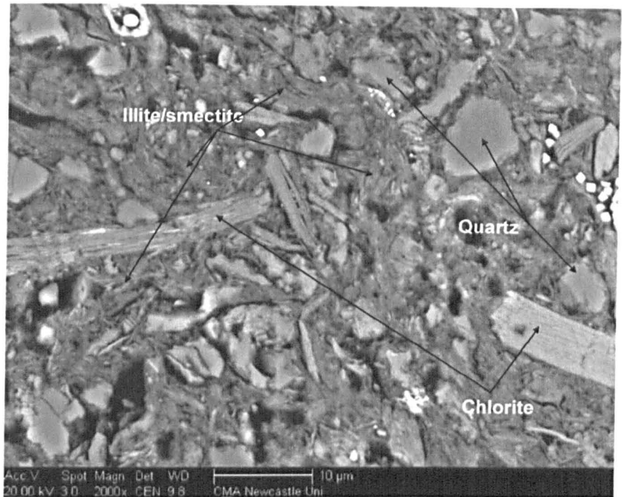
Figure 4.44. Magnus 1802.5[m] x 2000 magnification. Subround quartz grains surrounded by a variable matrix of phyllosilicate grains and groundmass below the resolution of the image. A large chlorite grain (arrowed) has undergone some replacement by pyrite and is probably detrital in origin. To the right of the quartz grain highlighted are small pyrite cubes. Areas of flocked illite/smectite are highlighted
