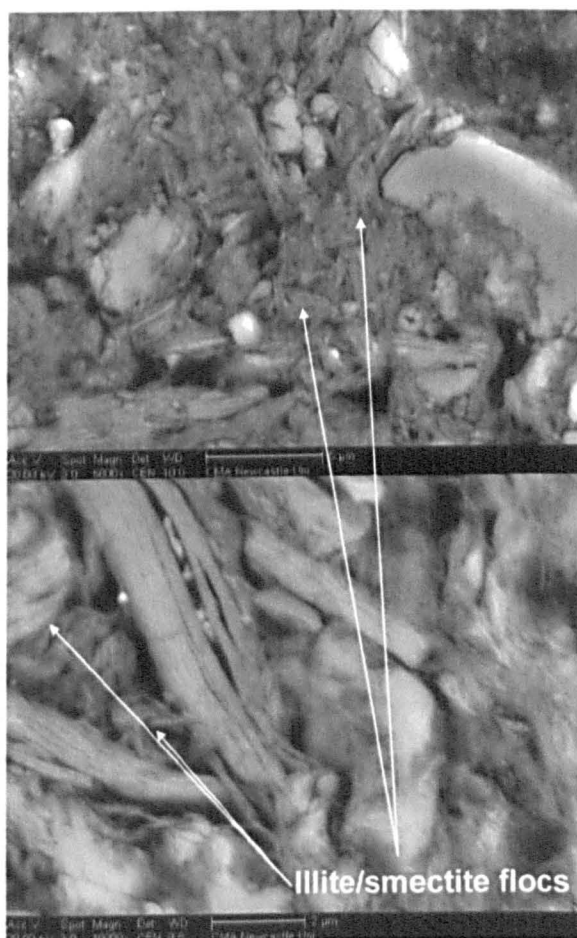
Figure 4.60. Samples from Magnus 211/12-2 at 1700m (top image) and 1802m (bottom image) at 5000x and 10000x magnification, respectively, showing the flocculation of illite/smectite particles persisting to present day burial depths.
