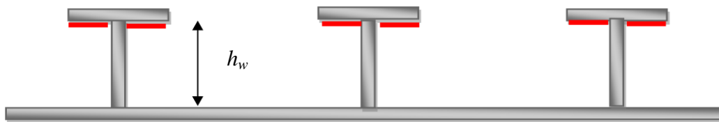
Figure 6-13 Stiffeners with web height less than d_{iso}
