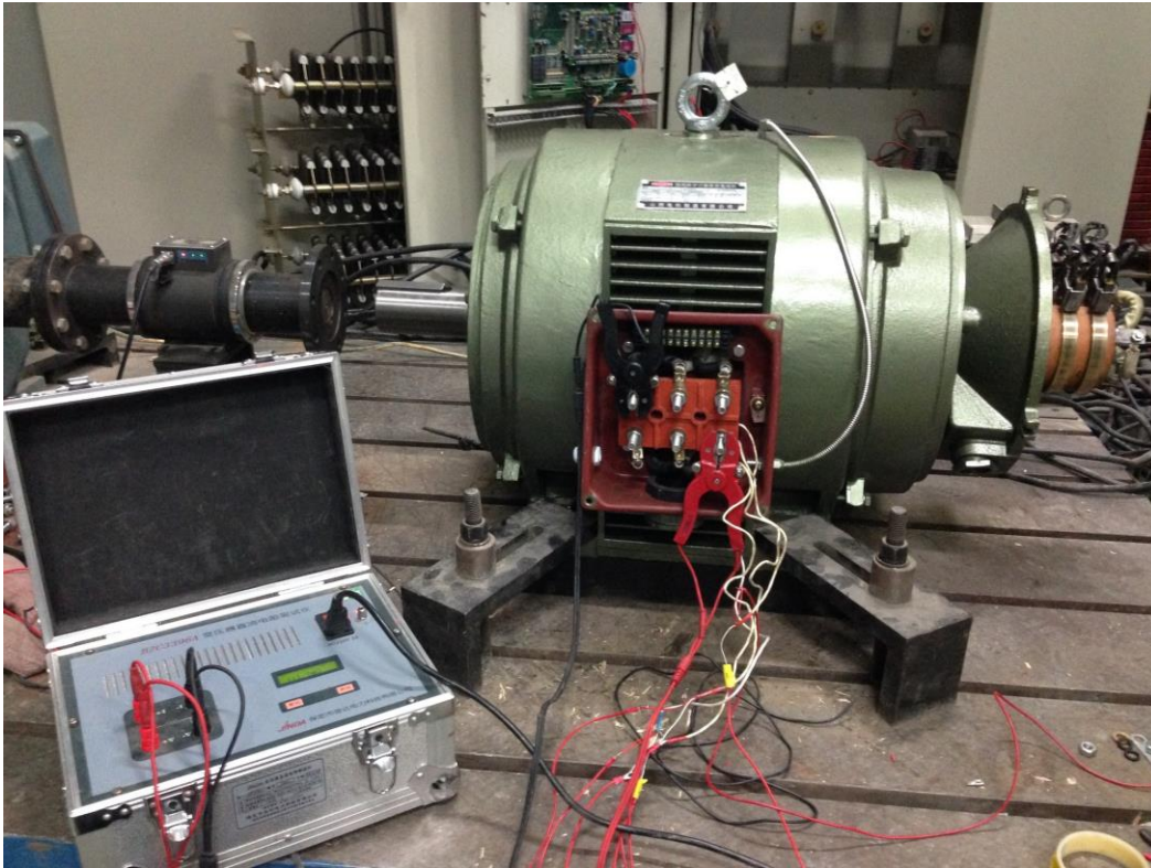
Figure C.1 Stator winding resistance measurement.
