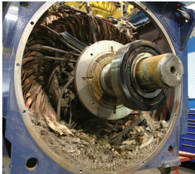
Figure 2.12 Catastrophic failure of a wind turbine generator due to rotor winding fault [43].
