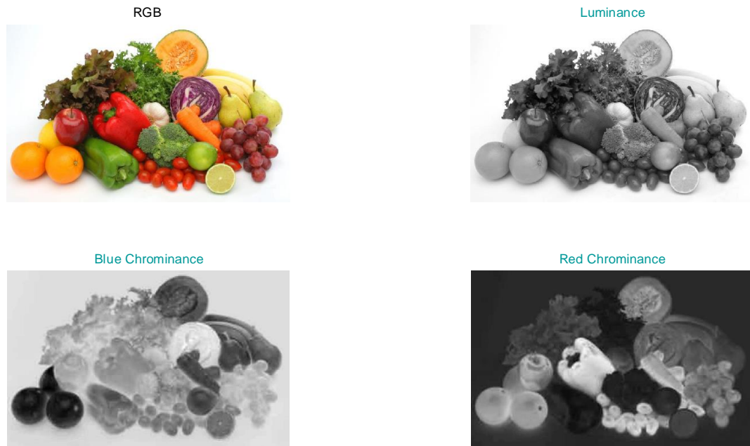
Figure 2.12 RGB image and the three colour channel intensity images of the YCbCr colour space
