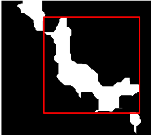
Figure 2.27 An example of a bounding box (in red) for a specific object
