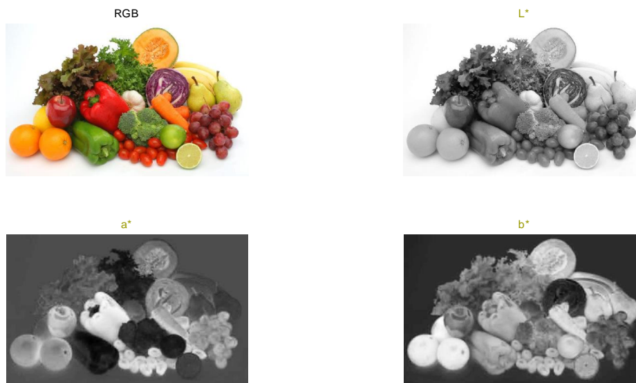
Figure 2.14 RGB image and the three colour channel intensity images of the L^*a^*b^* colour space
