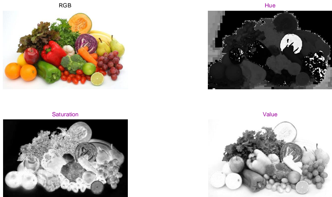
Figure 2.11 RGB image and the three colour channel intensity images of the HSV colourspace
