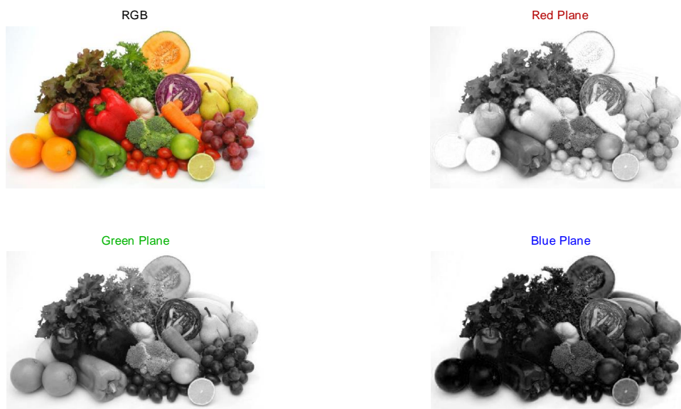
Figure 2.10 RGB image and the three colour channel intensity images of the RGB colourspace
