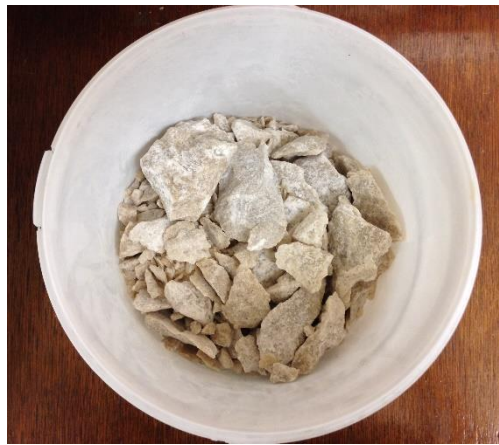
Figure 4-3 The salt hydrate S46 was supplied as solid chunks.
