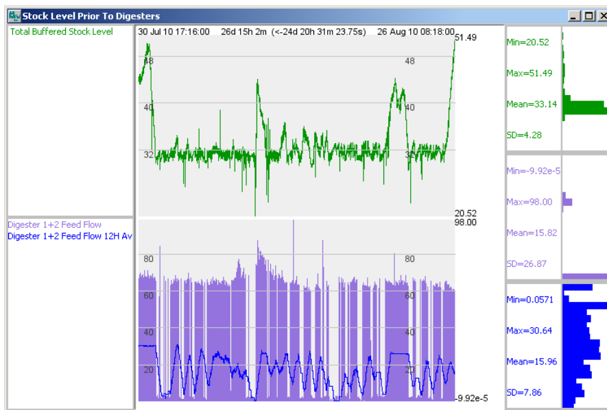
Figure 5.17 Sludge buffered stock level and digester feedflow
