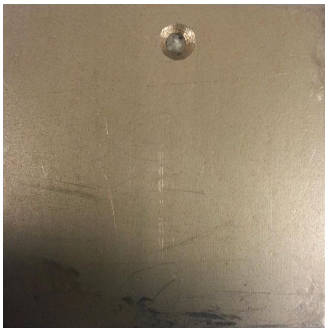
Figure 13: Photo of 5cmx5cm Coupon with Thin Film Remaining on Surface after Clean
