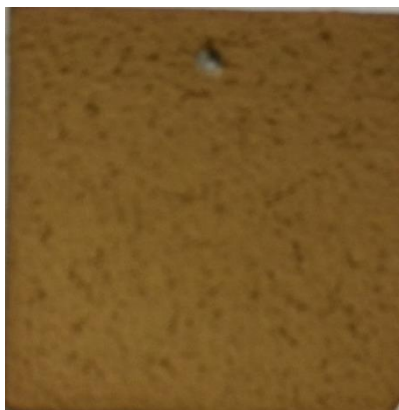
Figure 9: 5cmx5cm Fouled Coupon for Use on Bench Scale Cleaning Rig to Replicate Brewery Cleaning Scenario
