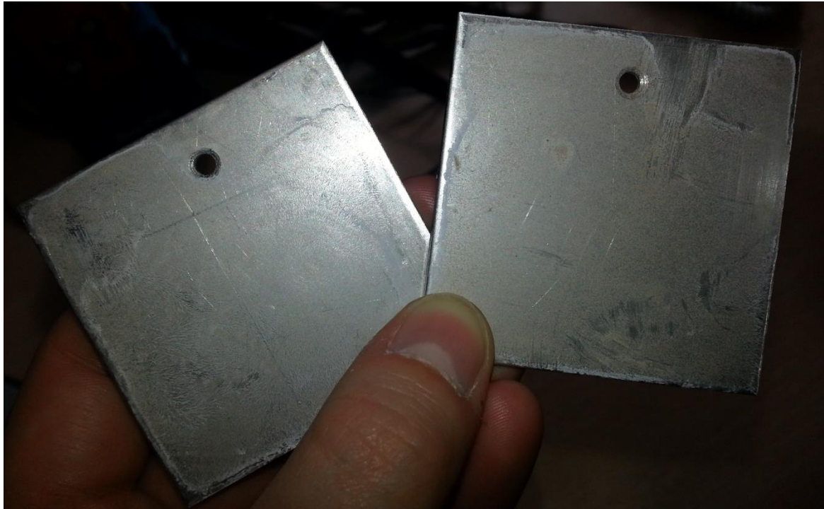
Figure 14: Photo of 5cmx5cm Coupons with Dried on White Powder Cake
