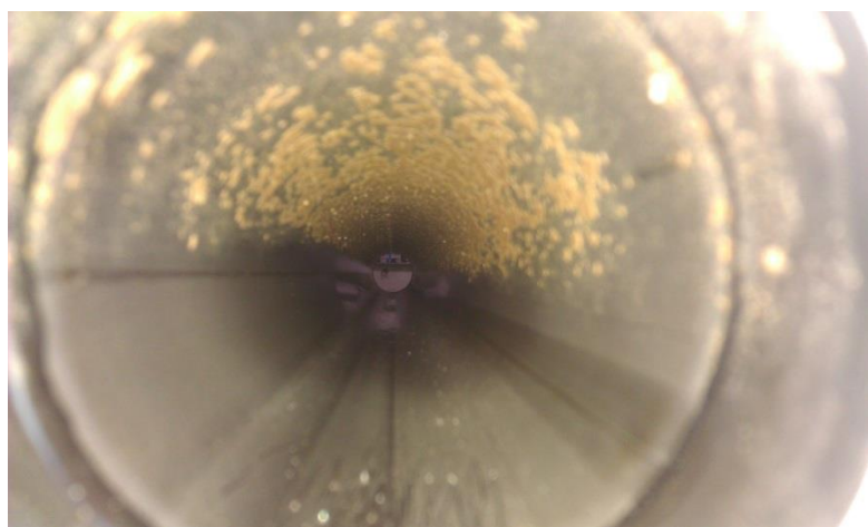
Figure 52: 2 inch Diameter Pipe with Top Half not cleaned after Experimental Cleaning Run
