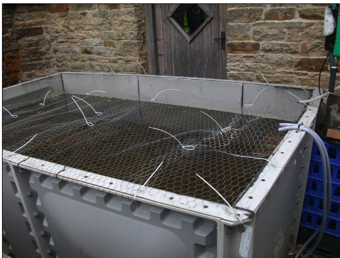
Figure 1.3 Nenthead compost-based pilot treatment system, note inlet pipes to right (photograph taken during spring 2012)
