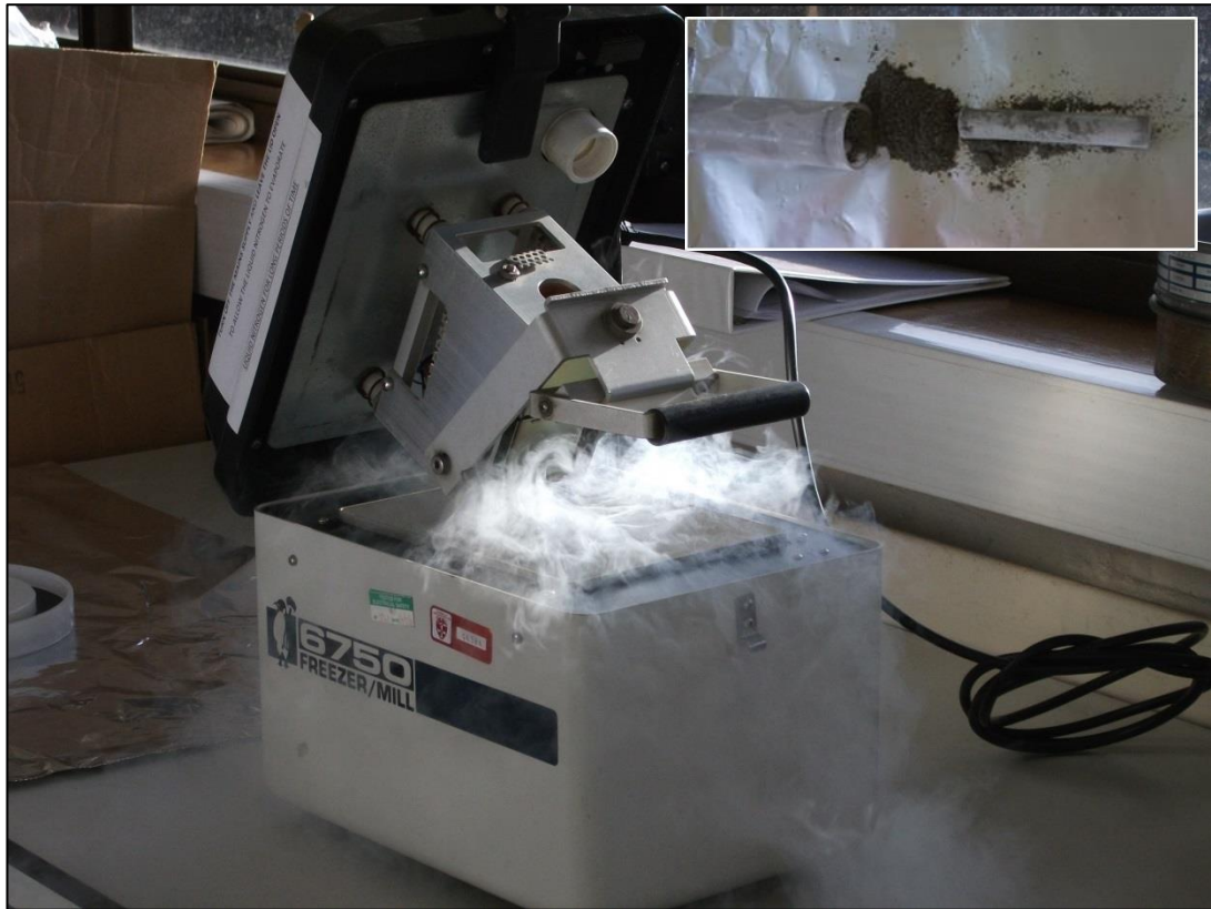
Figure 3.2 Spex™ liquid nitrogen pulveriser, inset showing pulverised substrate sample
