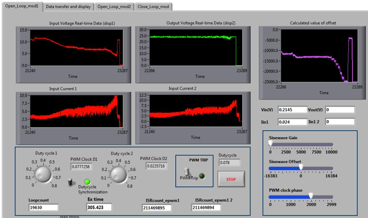
Figure 6.10 Part of the user's control panel in Labview
