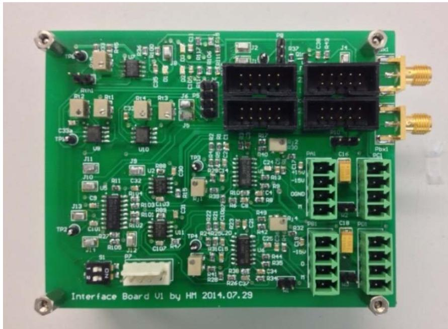
Figure 6.5 PWM generation board
