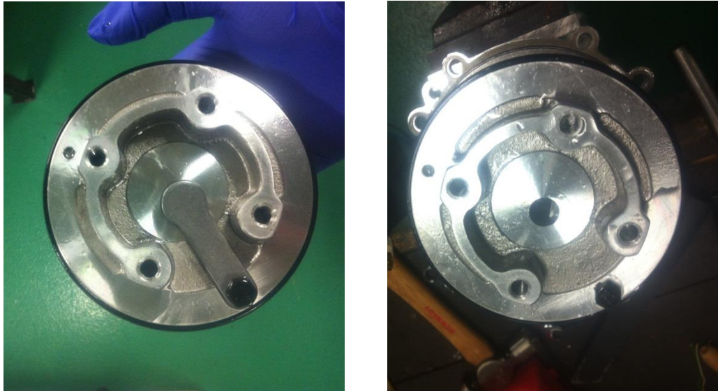
Figure 5-7 Removal process of the check valve from the stationary scroll (a) Stationary scroll with check valve (b) Stationary scroll without check valve
