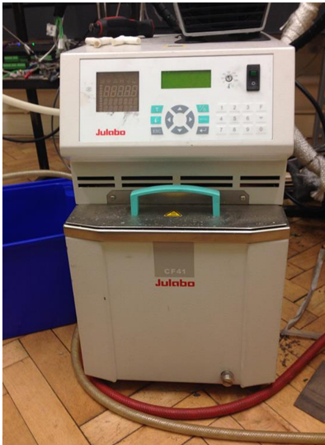
Figure 4-5 Picture of the cryostat for condenser/evaporator
