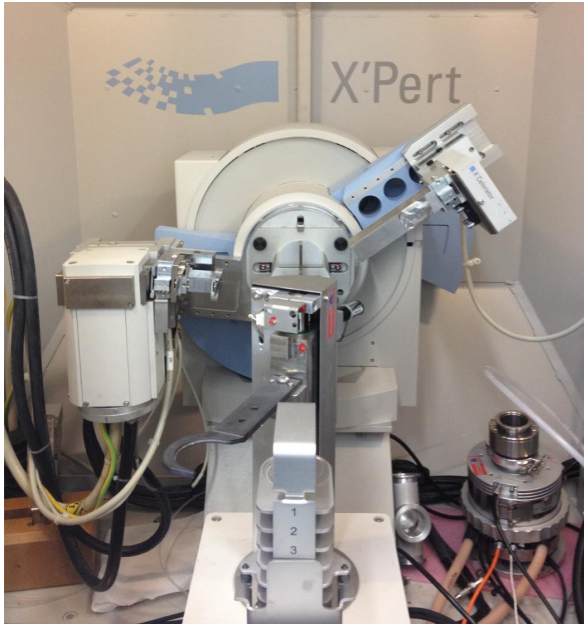
Figure 2.12 Photograph of the PANalytical X'Pert Pro MPD X-Ray diffractometer.
