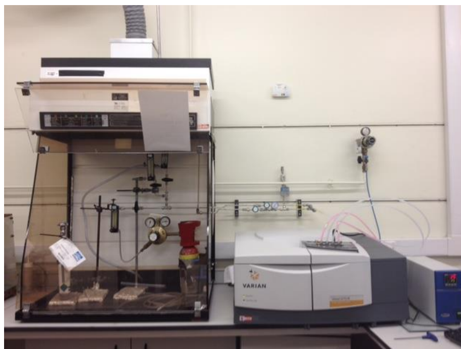
Figure 2.18 Photograph of the Varian 670-IR FTIR spectrometer.
