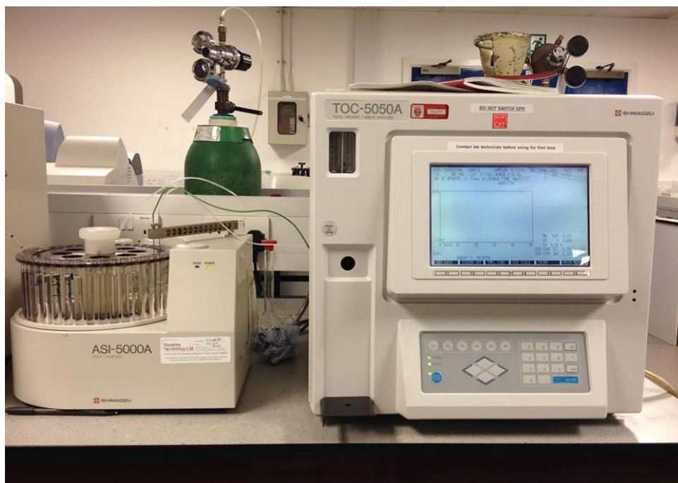
Figure 2.21 Photograph of the Shimadzu 5050A TOC analyser.
