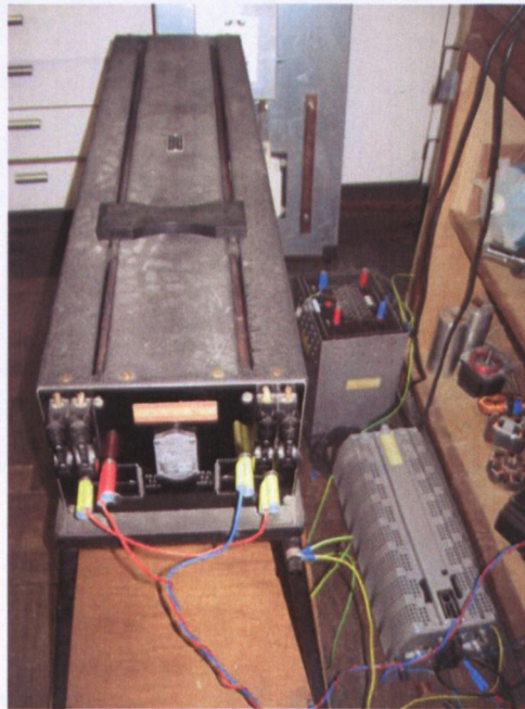
Figure D- 3- Freewheeling resistor, load resistor and isolation transformer
