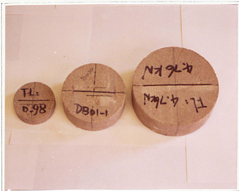
Photo 3.5 - Three CCNBD Specimens with Diameter 50, 75 and 100 mm
