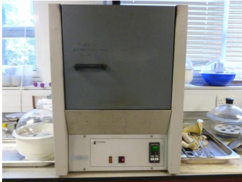
Figure 4-4 Furnace for volatile solids determination.
