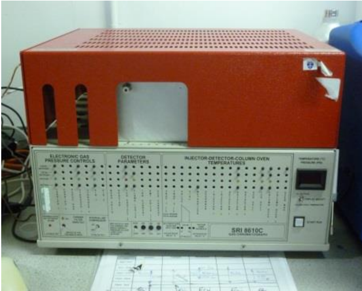
Figure 4-6 Gas chromatograph for methane content determination.
