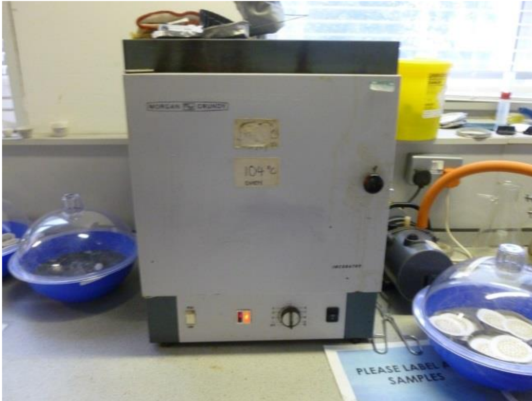
Figure 4-3 Oven used for Total Solids determination.
