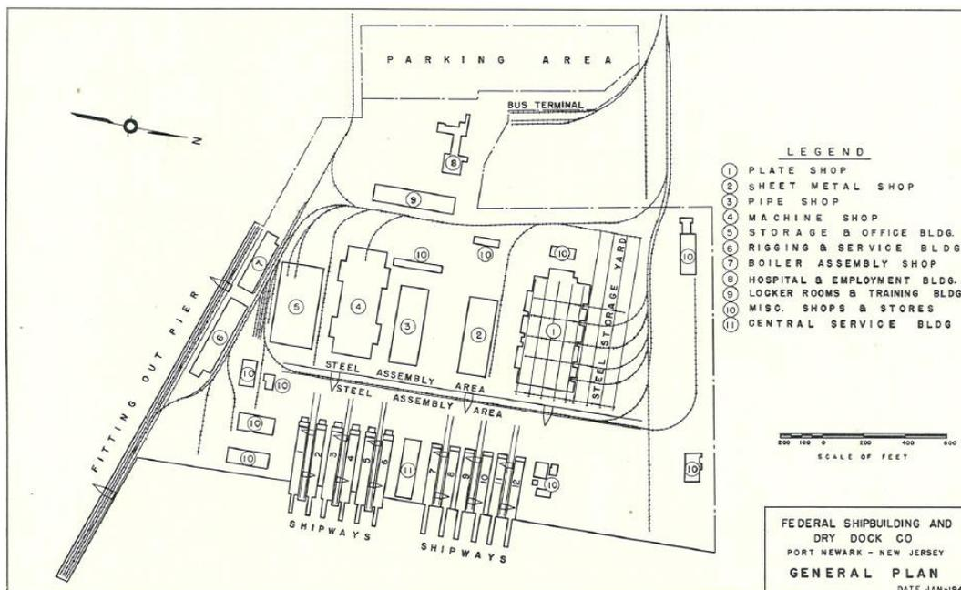
**Figure 2.3 - Arrangement of a WWII US shipyard showing slipway arrangements needed for capacity (Fassett, 1948, p. 243)**
