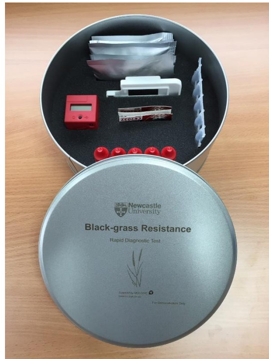
Figure 40 Prototype kit for Alopecurus myosuroides 'in-field' diagnostic. Kit designed and produced by Mologic Ltd (Bedfordshire, UK) contains enough for 5 tests to be carried out, a reader is also included this is the red box shown in the kit.
