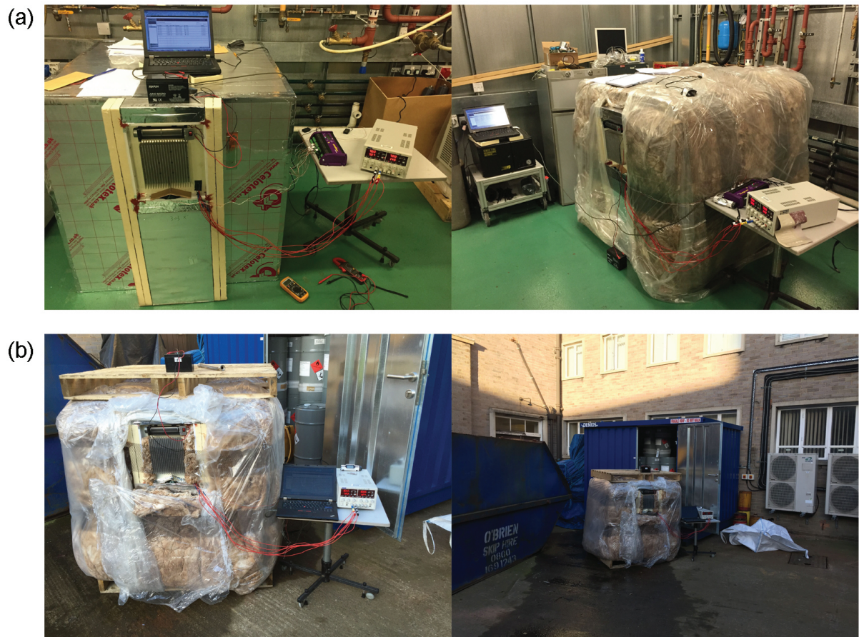
Fig. 3.7 Test ambient: (a) Heating test in lab ambient (b) Heating test in open-air courtyard ambient
