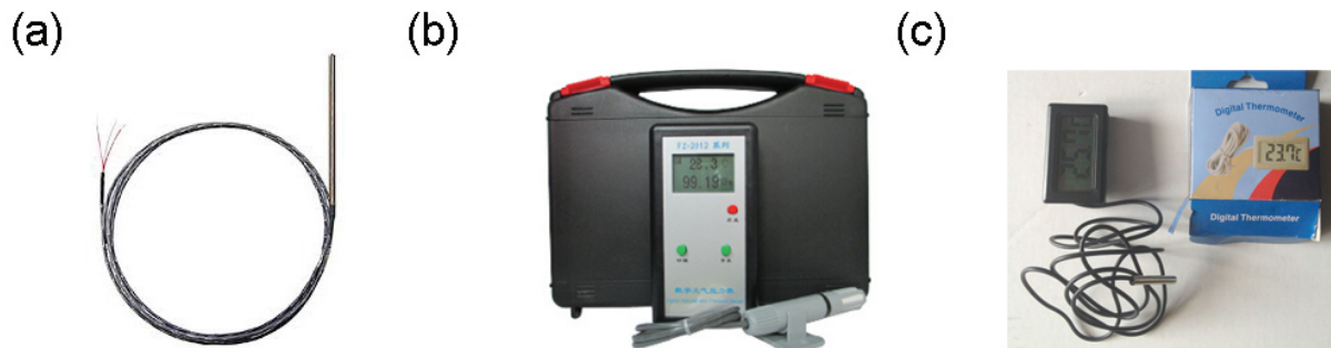
Fig. 3.4 Measurement devices: (a)PT100 RTD sensor (b)FZ-2012C digital air pressure, temperature and humidity monitor (c)TL8009 digital thermometer
