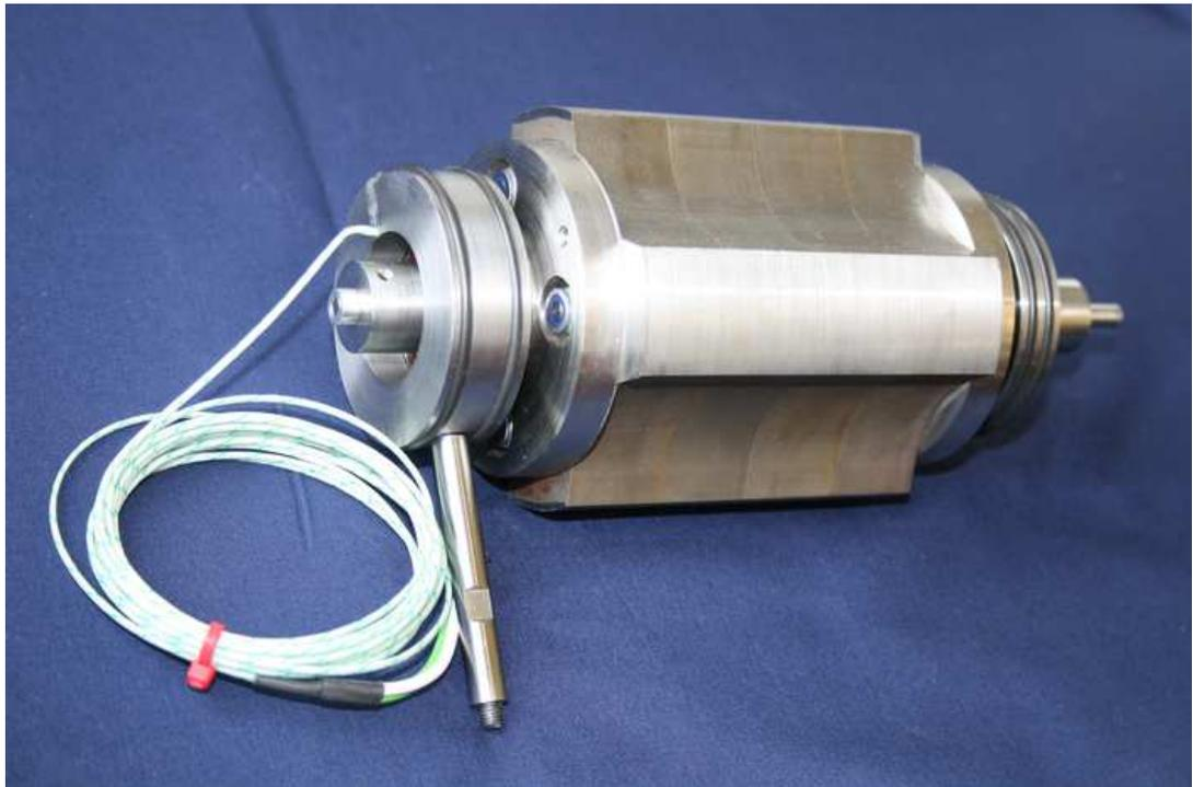
Figure 7.17: Fitted Magnet on the Rotor Shaft, Potted Thermocouple and Accelerometer Stud
