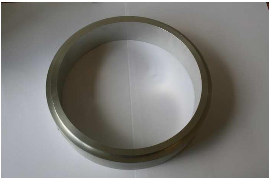
Figure 7.3: Stator Lamination Lock Ring
