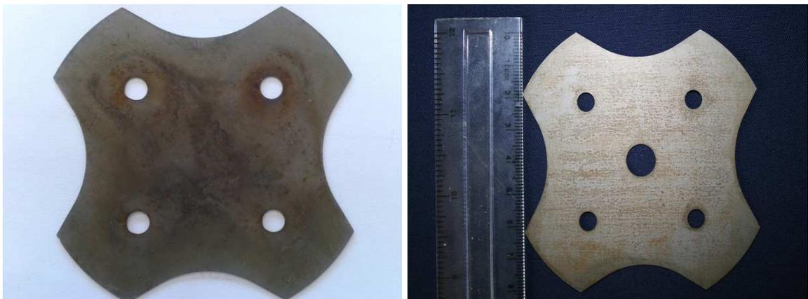
(a) Rotor Laminate without the Shaft Hole      (b) Rotor Laminate with a Shaft Hole
