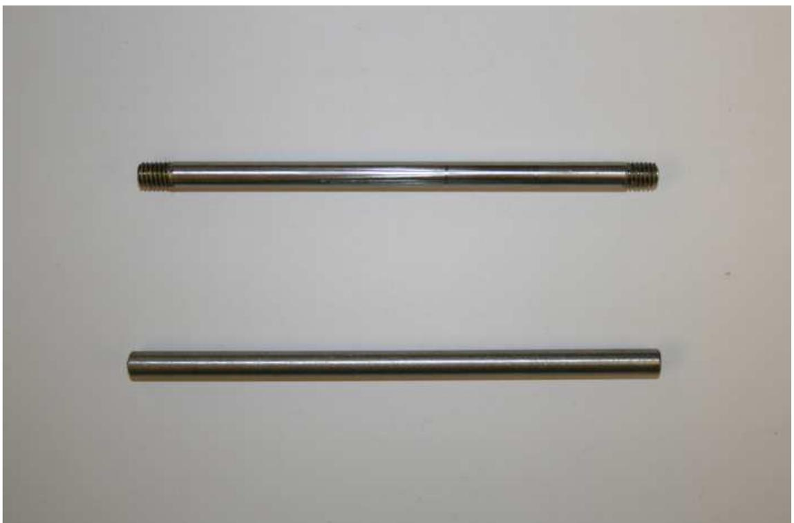
Figure 7.12: Rotor Tie Rods
