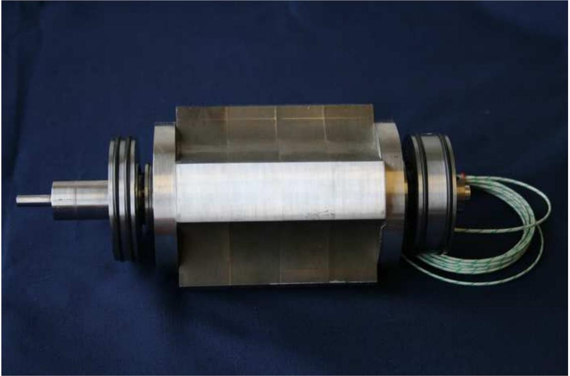
Figure 7.18: Fitted O’rings on the Bearing Cups
