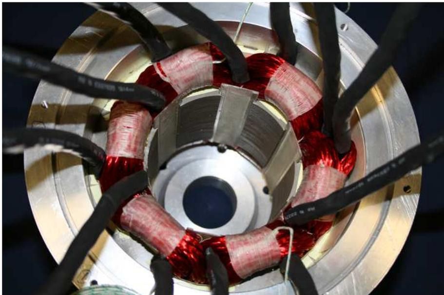
Figure 7.7: Tying Cords, Heat Shrinks and Thermal Coupling
