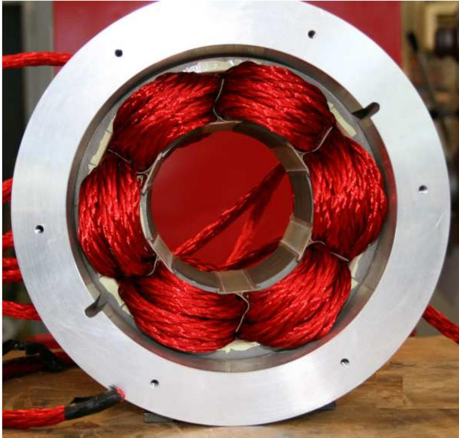
Figure 7.6: Coils, Nomex and Tufnol Insulations
