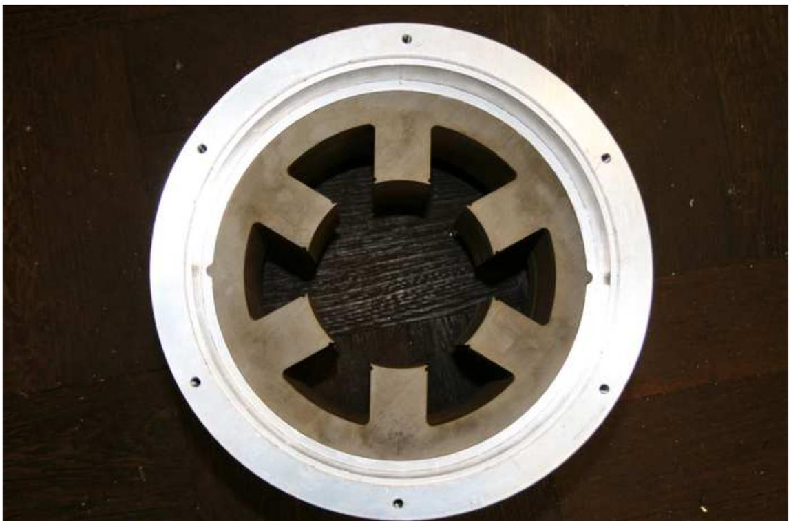
Figure A.2: Stator Inside the Case
