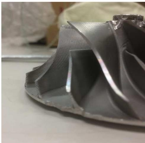
Figure 8.16: Evidence of Damage on the Compressor Wheel
