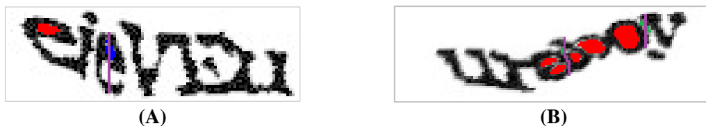
Figure 6.13. The loop segmentation errors: (A) In identifying the components and (B) in segmenting the components
