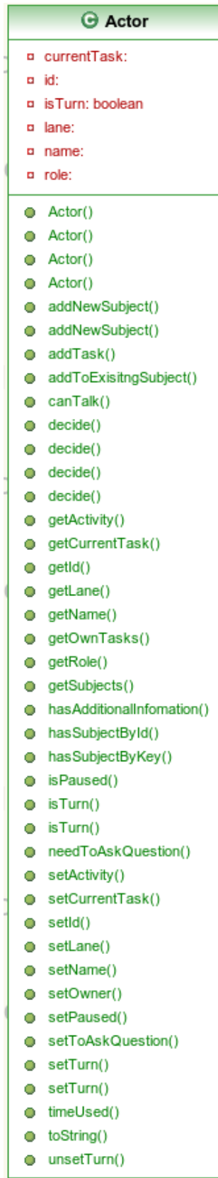
Figure 107: UML class diagram of complete Actor class
