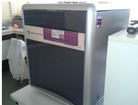
Figure 3.3. Elementar Vario Macro Cube for combustion method based nitrogen analysis.
