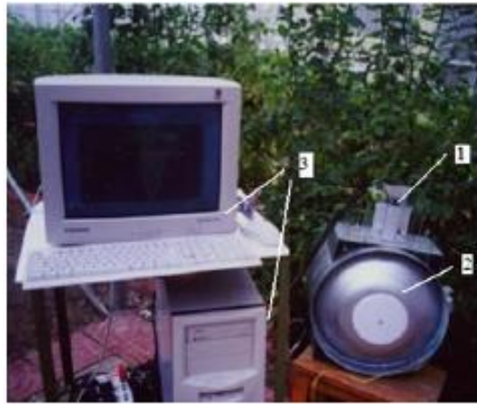
Figure 2.9. Image acquisition devices to identify nitrogen and potassium deficiency in tomato plants.
