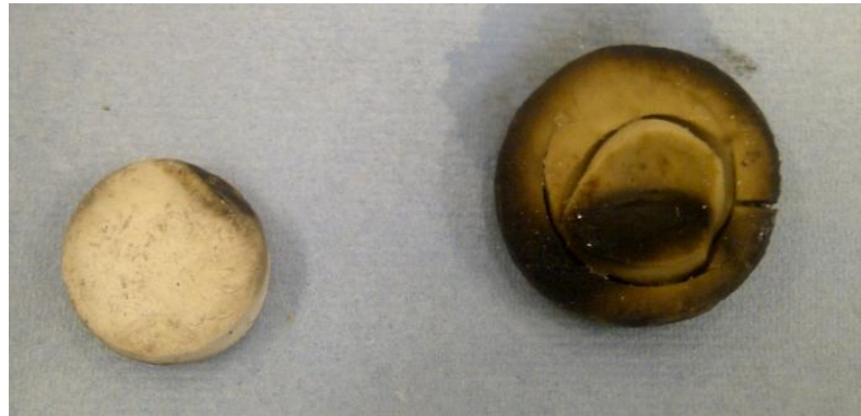
Figure 4-13 SPHPA10 swollen and cracked after water uptake test
