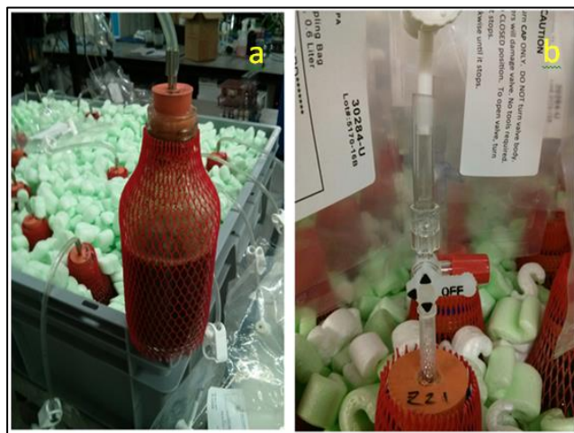
Fig. 3.3 Assembled reactors used in Batch Experiments 1 (a) and 2 (b)
