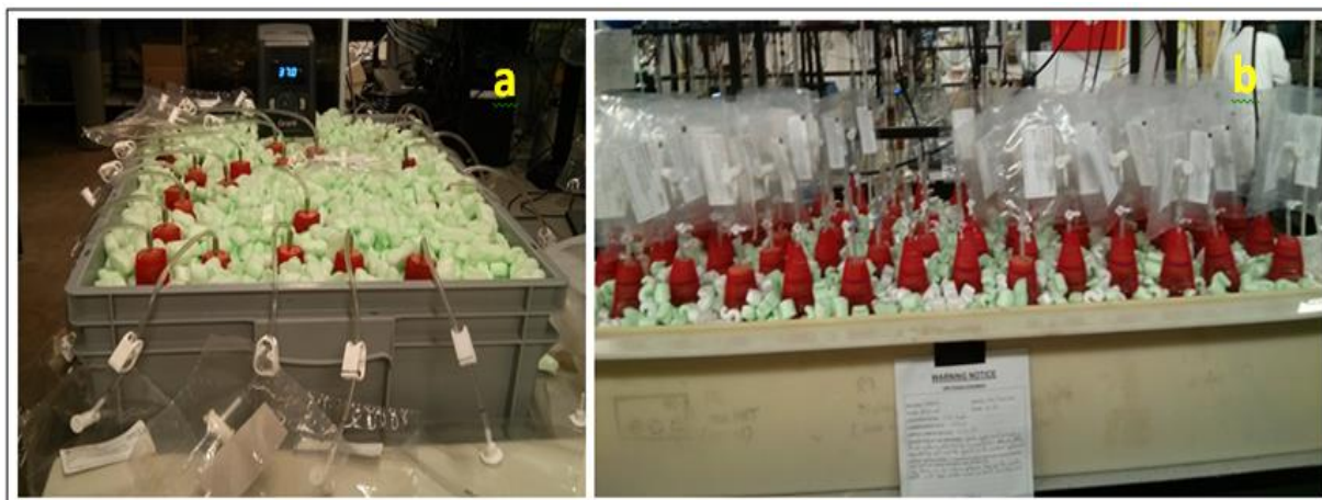
Fig. 3.5 Completed set up for (a) Experiment 1 and (b) Experiment 2, showing different gas take-off configurations and the use of polystyrene packing to prevent water evaporation.
