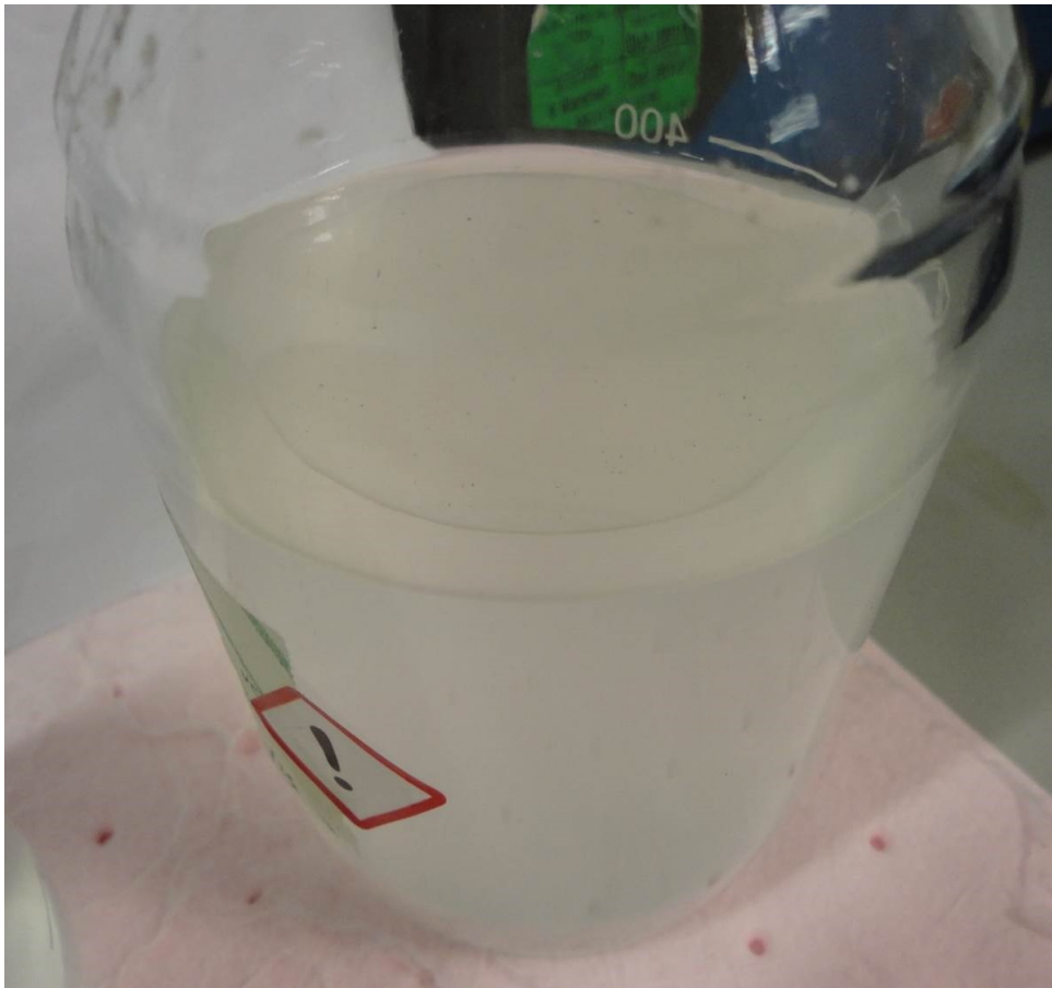
Figure 5.17: Aqueous phase after 120h perstraction with 1-heptanol. A layer of 1-heptanol can be observed on the surface of the synthetic ABE solution.
