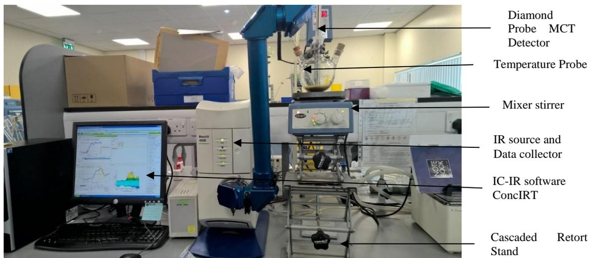
**Figure 3.4 FTIR On-line Monitoring of IST experimental setup**
