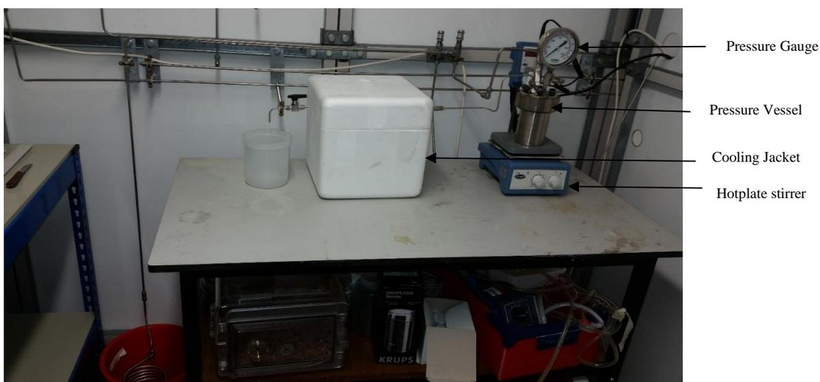
**Figure 3.6 Reactive coupling experimental rig**
