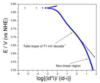
Figure 17: Tafel plot obtained for the Pd/C catalyst showing a single Tafel slope and a nonlinear region.
