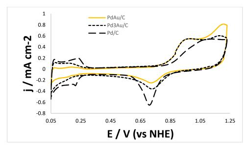
Figure 11: Cyclic voltammograms for PdAu/C, Pd<sub>3</sub>Au/C and Pd/C catalysts in N<sub>2</sub>-saturated 0.5 M H<sub>2</sub>SO<sub>4</sub> at a scan rate of 20 mVs<sup>-1</sup>.
