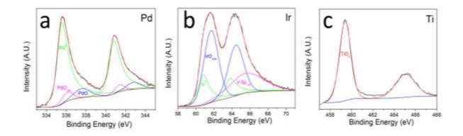
*Figure 54: Pd 3d, (labelled a) Ir 4f (labelled b) and Ti 2p (labelled c) XPS Spectra obtained for the PdIr/TiO<sub>2</sub>-C catalyst.*
