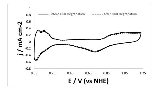
Figure 46: Cyclic voltammograms obtained for the commercial Pt/C catalyst before and after ORR degradation recorded at 20 mVs<sup>-1</sup> in N<sub>2</sub>-saturated H<sub>2</sub>SO<sub>4</sub>.
