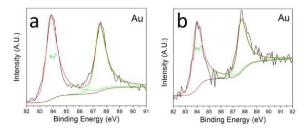
*Figure 42: Au 4f XPS Spectra obtained for PdIrAu/C before (labelled a) and after potential cycling (labelled b).*
