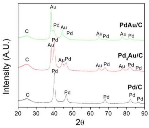
*Figure 5: X-ray diffraction patterns obtained for the Pd/C, Pd<sub>3</sub>Au/C and PdAu/C catalysts. Reflections labelled 'c, 'Pd' and 'Au' correspond to carbon, palladium and gold respectively.*
