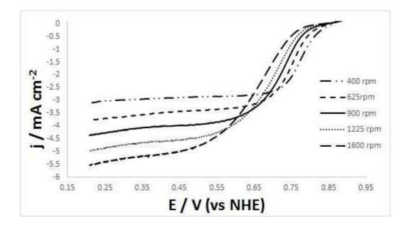
*Figure 14: Linear sweep voltammograms for commercial palladium (PdCOM) catalyst at a scan rate of 5 mVs<sup>-1</sup> and rotation rates of 400, 625, 900, 1225 and 1600 rpm.*
