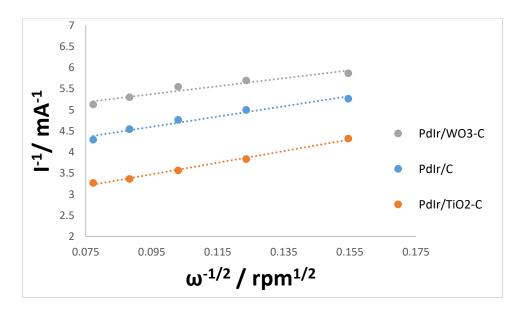
*Figure 58: Koutecky-Levich plots obtained for PdIr/C, PdIr/TiO<sub>2</sub>-C and PdIr/WO<sub>3</sub>-C catalysts.*
