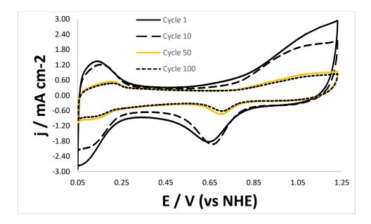
*Figure 62: First, tenth, fiftieth and hundredth cyclic voltammograms obtained for PdIr/TiO*<sub>2</sub>-*C catalyst during 100 cycles recorded at 100 mVs*<sup>-1</sup>.
