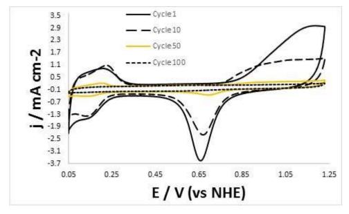
*Figure 23: First, tenth, fiftieth and hundredth cyclic voltammograms obtained for commercial 20 % palladium on carbon catalyst during 100 cycles recorded at 100 mVs<sup>-1</sup>.*
