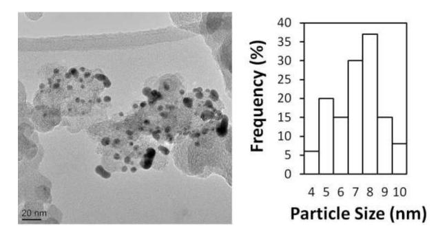
*Figure 8: TEM image obtained for PdAu/C and its corresponding particle size distribution showing a mixture of smaller and larger particles.*
