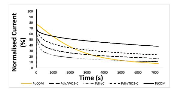
*Figure 67: Chronoamperometric response curves obtained for PdIr/TiO<sub>2</sub>-C, PdIr/WO<sub>3</sub>-C, PdIr/C, commercial Pd/C and Pt/C normalised to each catalyst's initial current.*
