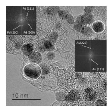
Figure 30: HRTEM image obtained for PdIrAu/C showing lattice planes of palladium and gold obtained on different particles.
