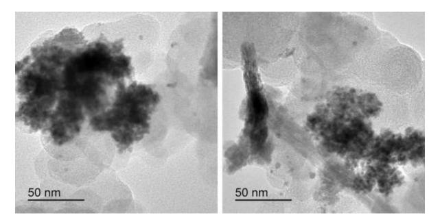
Figure 53: TEM image obtained for PdIr/WO<sub>3</sub>-C showing agglomeration.
