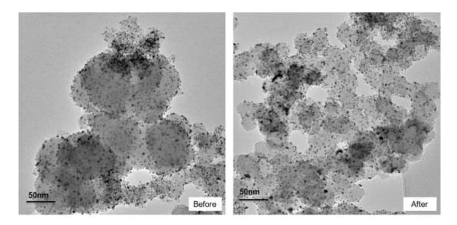
*Figure 49: TEM image obtained for commercial Pt/C before and after the ORR degradation in oxygen.*
