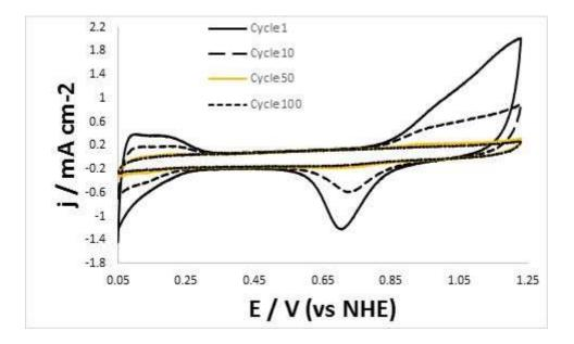
*Figure 19: First, tenth, fiftieth and hundredth cyclic voltammograms obtained for PdAu/C catalyst during 100 cycles recorded at 100 mVs<sup>-1</sup>.*
