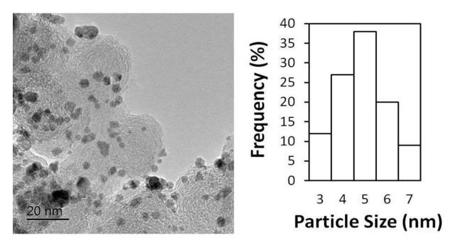
Figure 27: TEM image obtained for PdIr/C and its corresponding particle size distribution.
