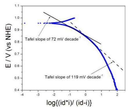
Figure 16: Tafel plot obtained for the commercial Pt/C catalyst showing two Tafel slopes of 72 and 119 mVdecade<sup>-1</sup>.
