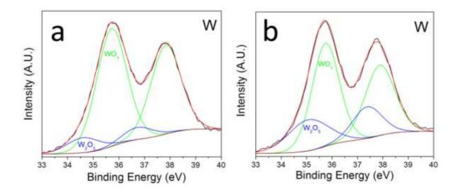
*Figure 66: W 4f XPS Spectra obtained for PdIr/WO<sub>3</sub>-C before (labelled a) and after potential cycling (labelled b).*
