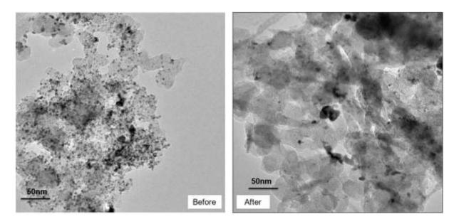
Figure 48: TEM image obtained for commercial Pd/C before and after the ORR degradation in oxygen.
