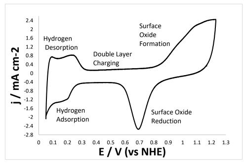
Figure 10: Cyclic voltammogram of Pd/C in  $N_2$ -saturated 0.5 M  $H_2SO_4$  at a scan rate of 100 mVs<sup>-1</sup>.
