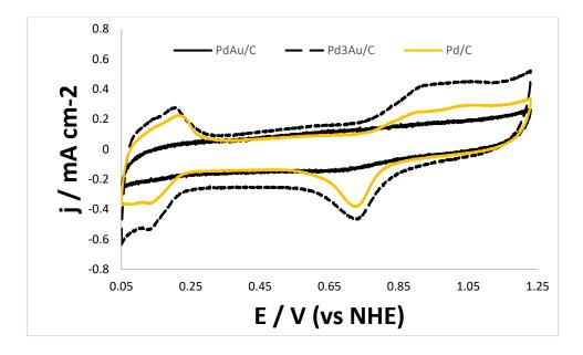
Figure 22: An overlay of the hundredth cyclic voltammogram obtained for PdAu/C,  $Pd_3Au/C$  and Pd/C catalysts recorded at 100 mVs<sup>-1</sup>.
