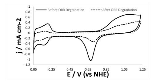
Figure 45: Cyclic voltammograms obtained for the commercial Pd/C catalyst before and after ORR degradation recorded at 20 mVs<sup>-1</sup> in  $N_2$ -saturated  $H_2SO_4$ .
