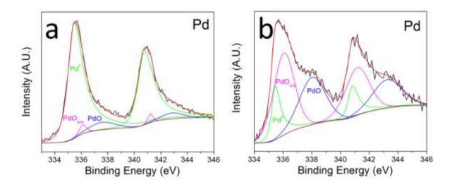
Figure 41: Pd 3d XPS Spectra obtained for PdIrAu/C before (labelled a) and after potential cycling (labelled b).
