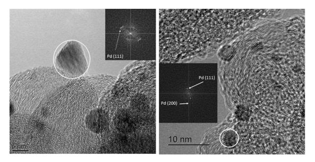
*Figure 29: High resolution image obtained for Pd/C and PdIr/C showing lattice planes for palladium.*
