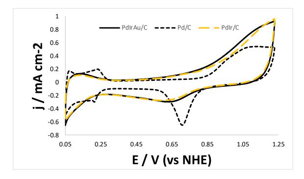
Figure 32: Cyclic voltammograms of Pd/C, PdIr/C and PdIrAu/C catalysts in  $N_2$ -saturated 0.5  $M H_2SO_4$  at a scan rate of 20 mVs<sup>-1</sup>.
