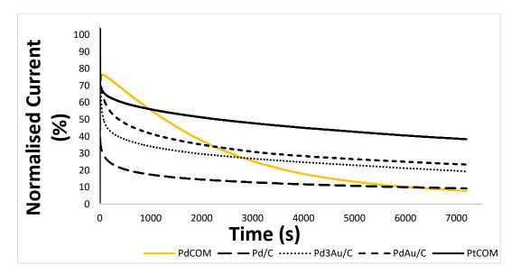
*Figure 25: Chronoamperometric response curves obtained for PdAu/C, Pd<sub>3</sub>Au/C, Pd/C, PdCOM and PtCOM catalysts based on normalising each catalyst's initial current to 100 %.*
