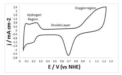
Figure 3: Cyclic voltammogram for a sample of prepared palladium on carbon catalyst, recorded in  $N_2$ -saturated 0.5 M H<sub>2</sub>SO<sub>4</sub> at a scan rate of 100 mVs<sup>-1</sup>.
