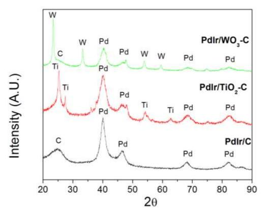
Figure 50: X-ray diffraction patterns obtained for PdIr/TiO<sub>2</sub>-C, PdIr/WO<sub>3</sub>-C and PdIr/C catalysts. Reflections labelled 'c, 'Ti' and 'W' correspond to carbon, titanium oxide and tungsten oxide respectively.
