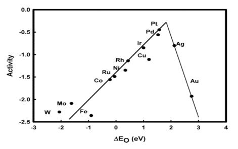
*Figure 1: Volcano plot showing trends in ORR activity as a function of oxygen binding energy* [20].
