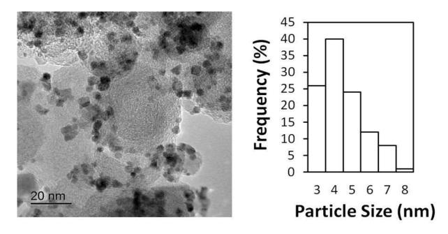
*Figure 51: TEM image for PdIr/TiO<sub>2</sub>-C and its corresponding particle size distribution.*
