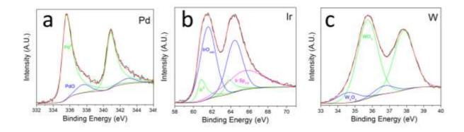
*Figure 55: Pd 3d (labelled a), Ir 4f (labelled b) and W 4f (labelled c) XPS Spectra obtained for the PdIr/WO<sub>3</sub>-C catalyst.*
