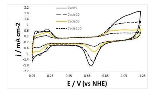
Figure 20: First, tenth, fiftieth and hundredth cyclic voltammograms obtained for  $Pd_3Au/C$  catalyst during 100 cycles recorded at 100 mVs<sup>-1</sup>.
