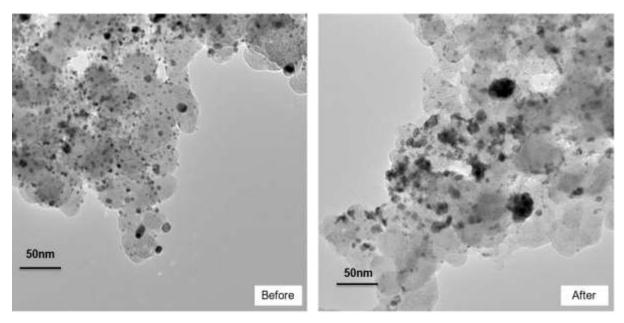
Figure 70: TEM image obtained for PdIr/C before and after the ORR degradation in oxygen.
