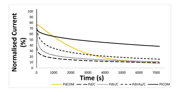
*Figure 43: Chronoamperometric response curves obtained PdIr/C, PdIrAu/C, Pd/C, commercial Pd/C and Pt/C catalysts normalised to each catalyst's initial current.*
