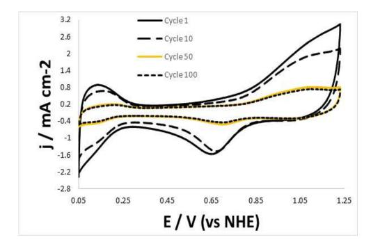
*Figure 37: First, tenth, fiftieth and hundredth cyclic voltammograms obtained for PdIr/C catalyst during 100 cycles recorded at 100 mVs<sup>-1</sup>.*
