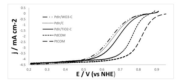
*Figure 57: Linear sweep voltammograms obtained for PdIr/TiO*<sub>2</sub>-*C, PdIr/WO*<sub>3</sub>-*C and PdIr/C compared with commercial Pd/C and Pt/C at 900 rpm and a scan rate of 5 mVs*<sup>-1</sup>.
