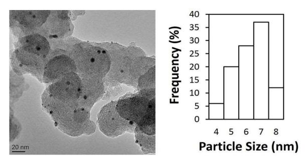
*Figure 7: TEM image obtained for Pd<sub>3</sub>Au/C and its corresponding particle size distribution showing well-dispersed particles.*
