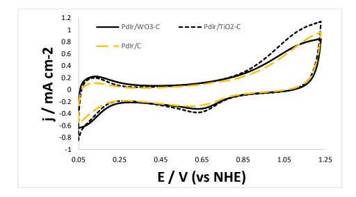
Figure 56: Cyclic voltammograms for PdIr/TiO<sub>2</sub>-C, PdIr/WO<sub>3</sub>-C and PdIr/C catalysts in  $N_2$  saturated 0.5 M H<sub>2</sub>SO<sub>4</sub> at scan rate 20 mVs<sup>-1</sup>.
