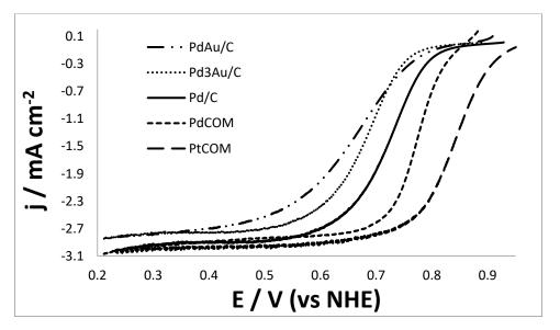
Figure 12: Linear sweep voltammograms for PdAu/C, Pd<sub>3</sub>Au/C and Pd/C compared with the commercial palladium and platinum at 400 rpm and scan rate of 5 mVs<sup>-1</sup>.
