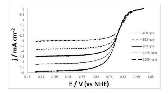
*Figure 15: Linear sweep voltammograms for commercial platinum (PtCOM) catalyst at a scan rate of 5 mVs<sup>-1</sup> and rotation rates of 400, 625, 900, 1225 and 1600 rpm.*
