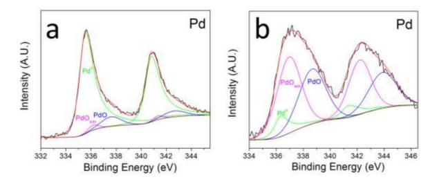
*Figure 39: Pd 3d XPS Spectra obtained for commercial Pd/C before (labelled a) and after potential cycling (labelled b).*
