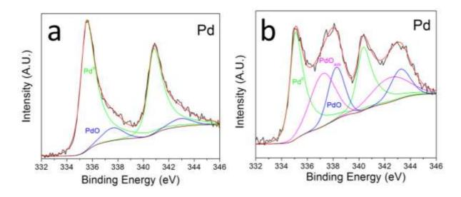
*Figure 64: Pd 3d XPS Spectra obtained for PdIr/WO<sub>3</sub>-C before (labelled a) and after potential cycling (labelled b).*
