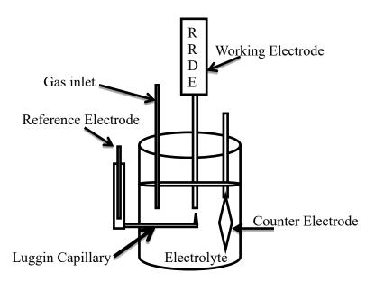
Figure 4: Schematic diagram of a 3-electrode cell.
