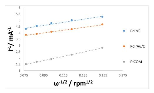
*Figure 34: Koutecky-Levich plots obtained for PdIr/C, PdIrAu/C and the commercial Pt/C catalyst at 0.67 V.*
