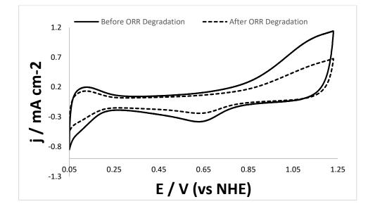
Figure 68: Cyclic voltammograms obtained for the PdIr/WO<sub>3</sub>-C catalyst before and after ORR degradation recorded at 20 mVs<sup>-1</sup> in N<sub>2</sub>-saturated H<sub>2</sub>SO<sub>4</sub>.
