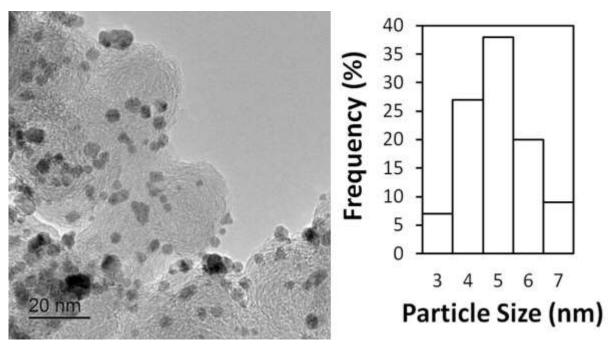
Figure 6: TEM image obtained for Pd/C and its corresponding particle size distribution showing particles of about 5 nm.
