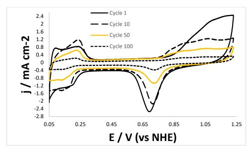
*Figure 21: First, tenth, fiftieth and hundredth cyclic voltammograms obtained for prepared Pd/C catalyst during 100 cycles recorded at 100 mVs<sup>-1</sup>.*
