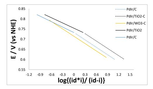
Figure 59: Tafel slopes for  $PdIr/TiO_2$ -C (2 slopes in black),  $PdIr/WO_3$ -C (single slope in yellow) and PdIr/C (2 slopes in blue).
