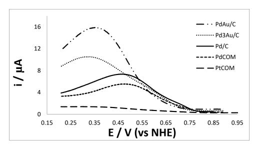
*Figure 18: Ring currents obtained for the PdAu/C, Pd<sub>3</sub>Au/C and Pd/C catalysts compared with the commercial palladium and platinum at 400 rpm and a scan rate of 5 mVs<sup>-1</sup>.*
