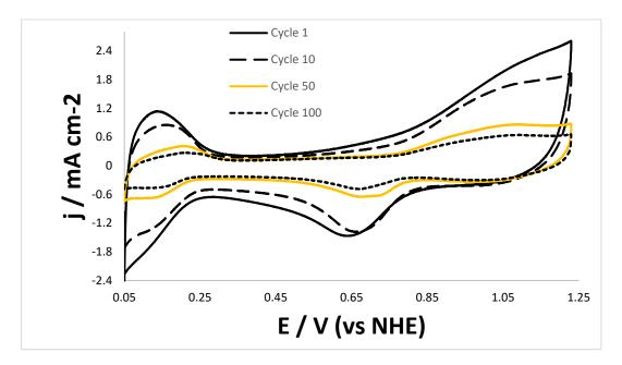
*Figure 38: First, tenth, fiftieth and hundredth cyclic voltammograms obtained for PdIrAu/C catalyst during 100 cycles recorded at 100 mVs<sup>-1</sup>.*
