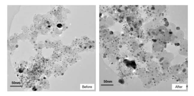
Figure 71: TEM image obtained for PdIr/TiO<sub>2</sub>-C before and after the ORR degradation in oxygen.
