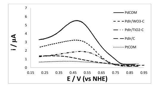
*Figure 60: Ring currents obtained for PdIr/TiO<sub>2</sub>-C, PdIr/WO<sub>3</sub>-C, PdIr/C, commercial Pd/C and Pt/C catalysts at 900 rpm.*
