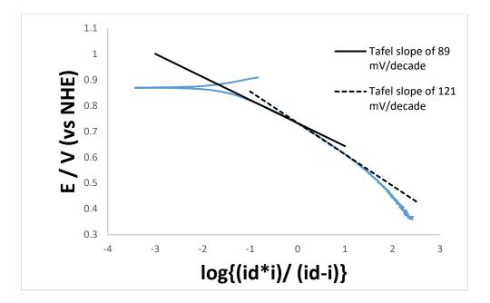
*Figure 35: Tafel plot obtained for the PdIr/C catalyst showing its two Tafel slopes of 89 and 121 mVdecade<sup>-1</sup> at the low and high current density regions respectively.*
