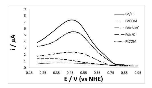
*Figure 36: Ring currents obtained for PdIr/C, PdIrAu/C, Pd/C, commercial Pd/C and commercial Pt/C catalysts at 900 rpm and a scan rate of 5 mVs<sup>-1</sup>.*
