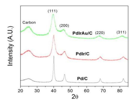
Figure 26: X-ray diffraction patterns obtained for PdIr/C, PdIrAu/C and Pd/C catalysts.
