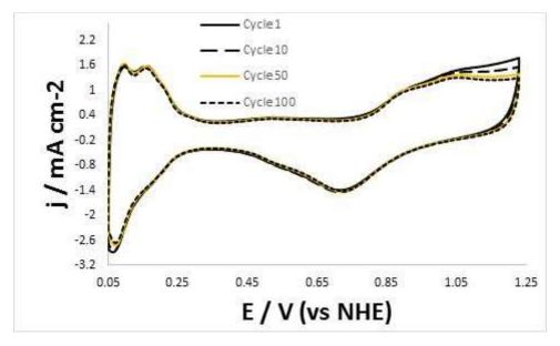
*Figure 24: First, tenth, fiftieth and hundredth cyclic voltammograms obtained for commercial 20 % platinum on carbon catalyst during 100 cycles recorded at 100 mVs<sup>-1</sup>.*
