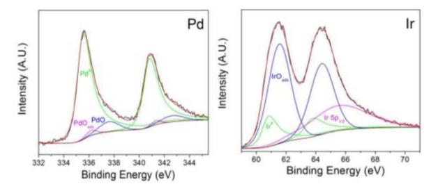
Figure 31: Pd 3d and Ir 4f XPS Spectra obtained for PdIr/C.
