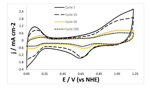
*Figure 61: First, tenth, fiftieth and hundredth cyclic voltammograms for PdIr/WO<sub>3</sub>-C catalyst during 100 cycles recorded at 100 mVs<sup>-1</sup>.*
