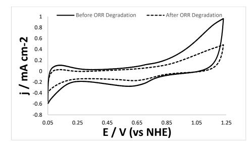
*Figure 44: Cyclic voltammograms obtained for the PdIr/C catalyst before and after ORR degradation recorded at 20 mVs<sup>-1</sup> in N<sub>2</sub>-saturated H<sub>2</sub>SO<sub>4</sub>.*
