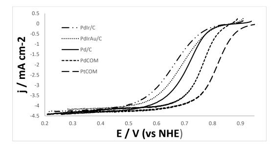
*Figure 33: Linear sweep voltammograms for PdIr/C, PdIrAu/C compared with Pd/C, commercial Pd/C and commercial Pt/C at 900 rpm and a scan rate of 5 mVs<sup>-1</sup>.*
