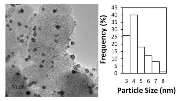
Figure 28: TEM image obtained for PdIrAu/C and its corresponding particle size distribution.
