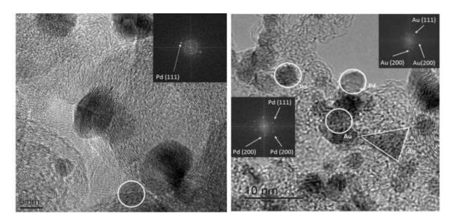
*Figure 9: High resolution image obtained for Pd/C and Pd<sub>3</sub>Au/C showing lattice planes for palladium and gold.*
