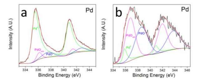
*Figure 40: Pd 3d XPS Spectra obtained for PdIr/C before (labelled a) and after potential cycling (labelled b).*
