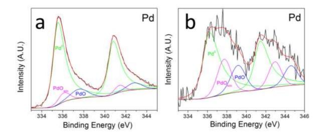
*Figure 63: Pd 3d XPS Spectra obtained for PdIr/TiO*<sub>2</sub>-*C before (labelled a) and after potential cycling (labelled b).*
