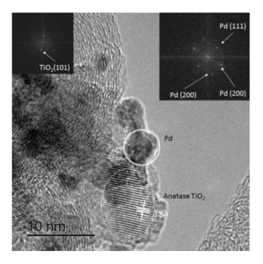
Figure 52: High resolution image obtained for  $PdIr/TiO_2$ -C showing lattice planes and the close interaction between palladium and  $TiO_2$ .
