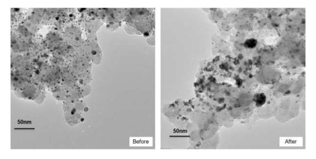
Figure 47: TEM image obtained for PdIr/C before and after the ORR degradation in oxygen.
