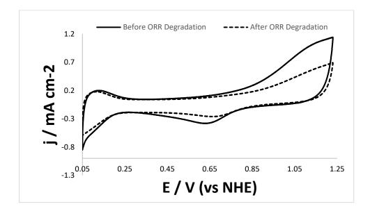
Figure 69: Cyclic voltammograms obtained for the PdIr/TiO<sub>2</sub>-C catalyst before and after ORR degradation recorded at 20 mVs<sup>-1</sup> in  $N_2$ -saturated  $H_2SO_4$ .
