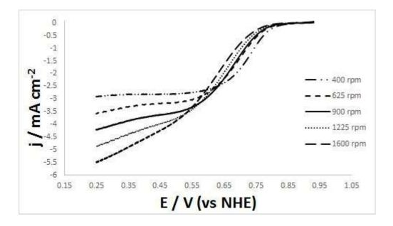
Figure 13: Linear sweep voltammograms for Pd/C catalyst at a scan rate of 5 mVs<sup>-1</sup> and rotation rates of 400, 625, 900, 1225 and 1600 rpm.
