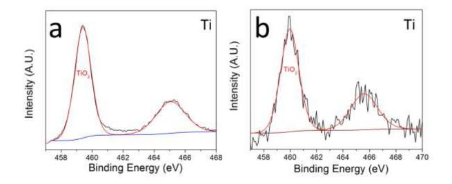
Figure 65: Ti 2p XPS Spectra obtained for PdIr/TiO2-C before (labelled a) and after potential cycling (labelled b).
