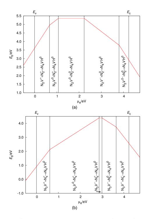
Figure 11.26: a) The reaction between a  $N_2V$  and  $N_2$  defect and b) the reaction between a  $N_3V$  and  $N_s$  defect, both form the  $N_4V$  centre, further details are listed in Figure 11.4.
