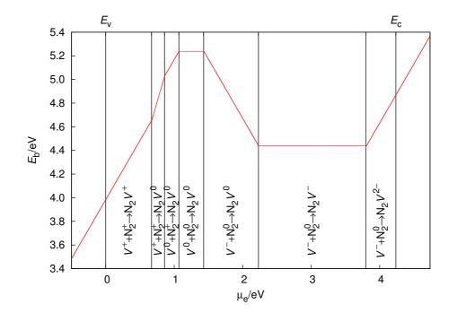
The binding energy for this reaction ranges from around 4.0–5.2 eV (Figure 11.10).
