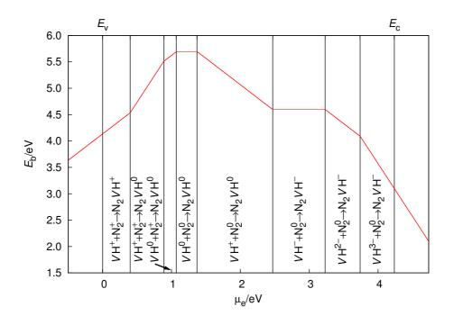
Figure 11.16: The reaction between a VH and  $N_2$  defect to form the  $N_2VH$  centre, further details are listed in Figure 11.4.
