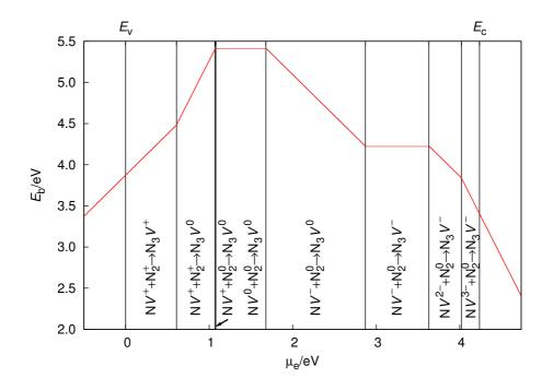
Figure 11.18: The reaction between a NV and  $N_2$  defect to form the  $N_3V$  centre, further details are listed in Figure 11.4.
