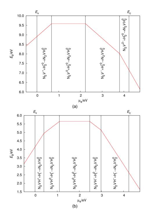
Figure 11.22: a) The reaction between a  $N_2V$  and  $H_2^*$  defect and b) the reaction between a  $N_2VH$  and  $H_i$  defect, both form the  $N_2VH_2$  centre, further details are listed in Figure 11.4.
