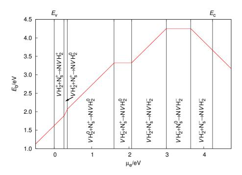
Figure 11.14: The reaction between a  $VH_2$  and  $N_s$  defect to form the N $VH_2$  centre, further details are listed in Figure 11.4.
