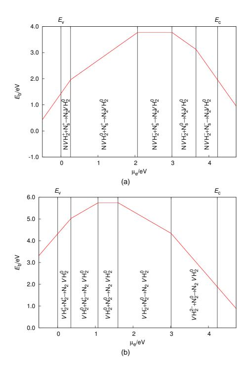
Figure 11.23: a) The reaction between a  $NVH_2$  and  $N_s$  defect and b) the reaction between a  $VH_2$  and  $N_2$  defect, both form the  $N_2VH_2$  centre, further details are listed in Figure 11.4.
