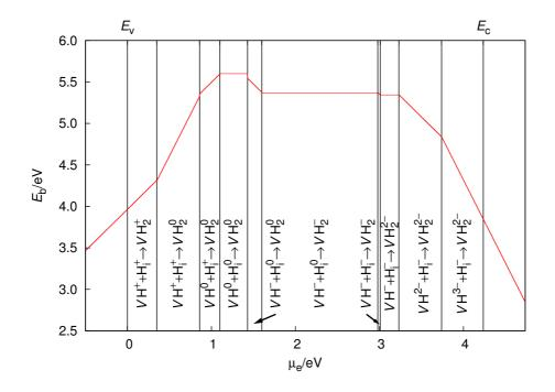
Figure 11.7: The reaction between VH and  $H_i$  defect to form the VH<sub>2</sub> centre, further details are listed in Figure 11.4.
