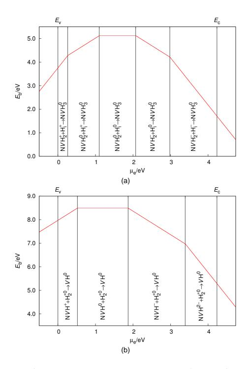
Figure 11.21: a) The reaction between a  $NVH_2$  and  $H_i$  defect and b) the reaction between a NVH and  $H_2^*$  defect, both form the  $NVH_3$  centre, further details are listed in Figure 11.4.
