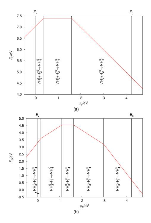
Figure 11.19: a) The reaction between a  $VH_2$  and  $H_2^*$  defect and b) the reaction between a  $VH_3$  and  $H_i$  defect, both form the  $VH_4$  centre, further details are listed in Figure 11.4.
