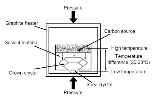
Figure 1.5: A schematic of HPHT apparatus. (Image after [31, p. 9]).
