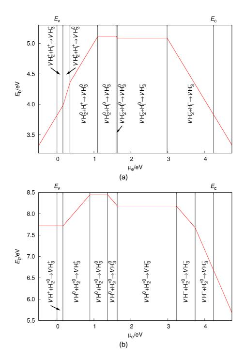
Figure 11.12: a) The reaction between a  $VH_2$  and  $H_i$  defect and b) the reaction between a VH and  $H_2^*$  defect, both form the  $VH_3$  centre, further details are listed in Figure 11.4.
