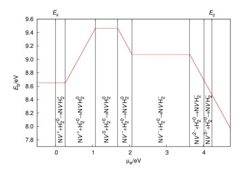
Figure 11.13: The reaction between a NV and  $H_2^*$  defect to form the NVH<sub>2</sub> centre, further details are listed in Figure 11.4.
