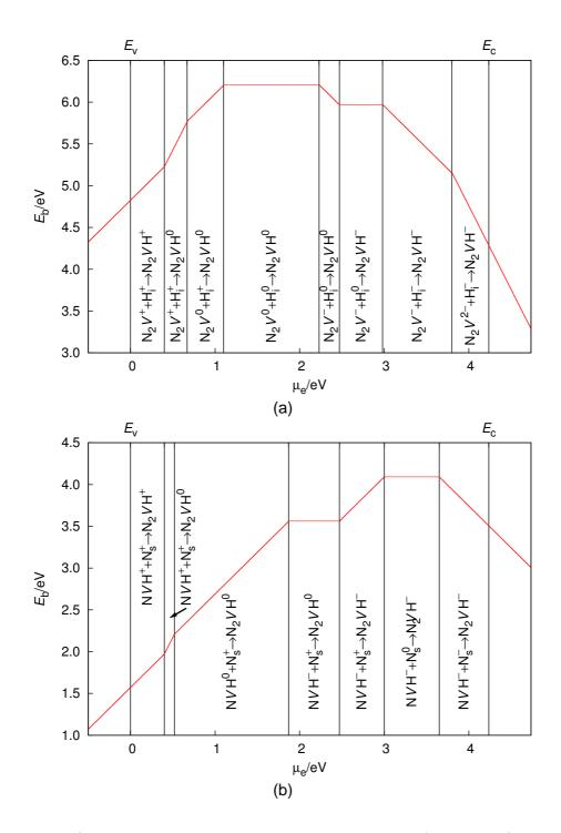
Figure 11.15: a) The reaction between a  $N_2V$  and  $H_i$  defect and b) the reaction between a NVH and  $N_s$  defect, both form the  $N_2VH$  centre, further details are listed in Figure 11.4.
