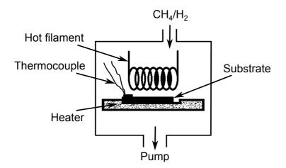
Figure 1.6: Hot filament CVD apparatus setup. (Image after [37]).
