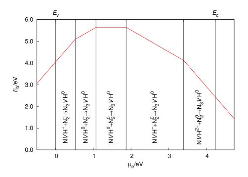
Figure 11.25: The reaction between a NVH and  $N_2$  defect to form the  $N_3VH$  centre, further details are listed in Figure 11.4.
