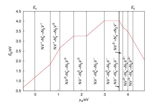
Figure 11.11: The reaction between a NV and  $N_s$  defect to form the  $N_2V$  centre, further details are listed in Figure 11.4.
