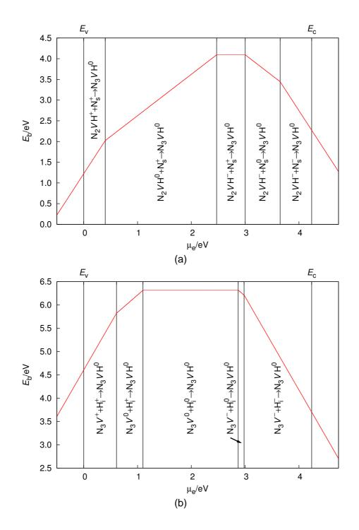
Figure 11.24: a) The reaction between a  $N_2VH$  and  $N_s$  defect and b) between a  $N_3V$  and  $H_i$  defect to form the  $N_3VH$  defect, further details are listed in Figure 11.4.
