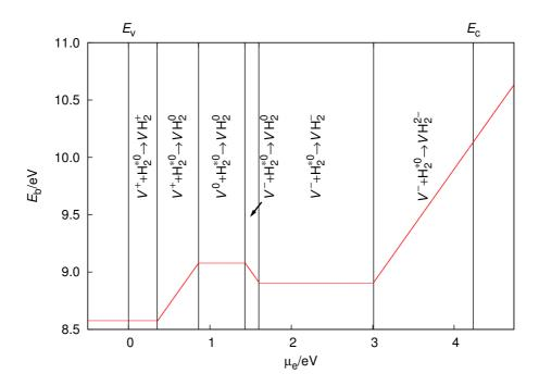
Figure 11.6: The reaction between a V and  $H_2^*$  defect to form the VH<sub>2</sub> centre, further details are listed in Figure 11.4.
