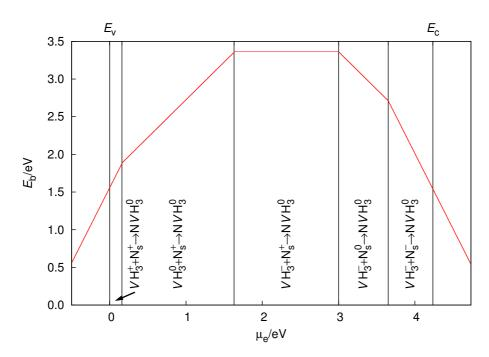
Figure 11.20: The reaction between a  $VH_3$  and  $N_s$  defect to form the NVH<sub>3</sub> centre, further details are listed in Figure 11.4.
