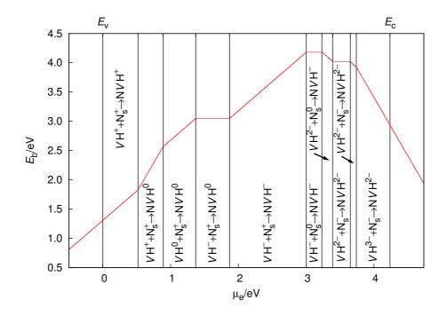
Figure 11.9: The reaction between a VH and  $N_s$  defect to form the NVH centre, further details are listed in Figure 11.4.
