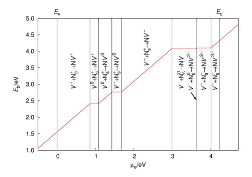
Figure 11.5: The reaction between a V and  $N_s$  to form the NV centre, further details are listed in Figure 11.4.
