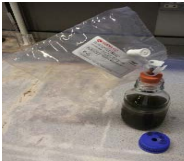
Figure 4-2. Modified BMP reactor and gas collection bag
