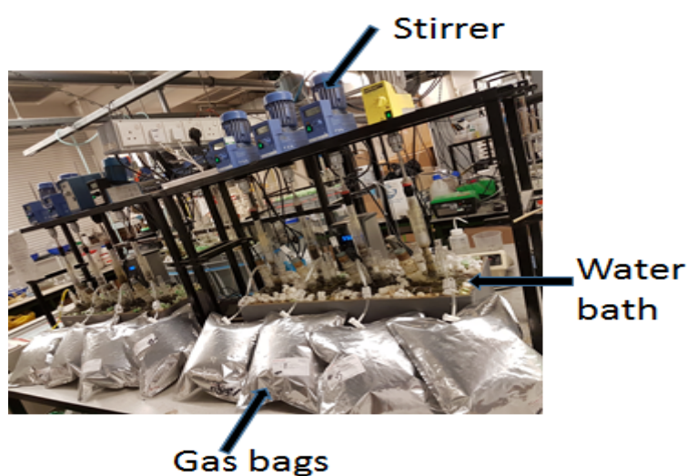
Figure 3-2 Continuous reactor set up and design
