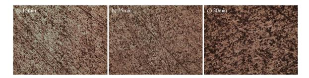
Figure 5.5: Aluminium surfaces after: a) 15min, b) 25min and c) 30min of anodising (OM - 10x).
