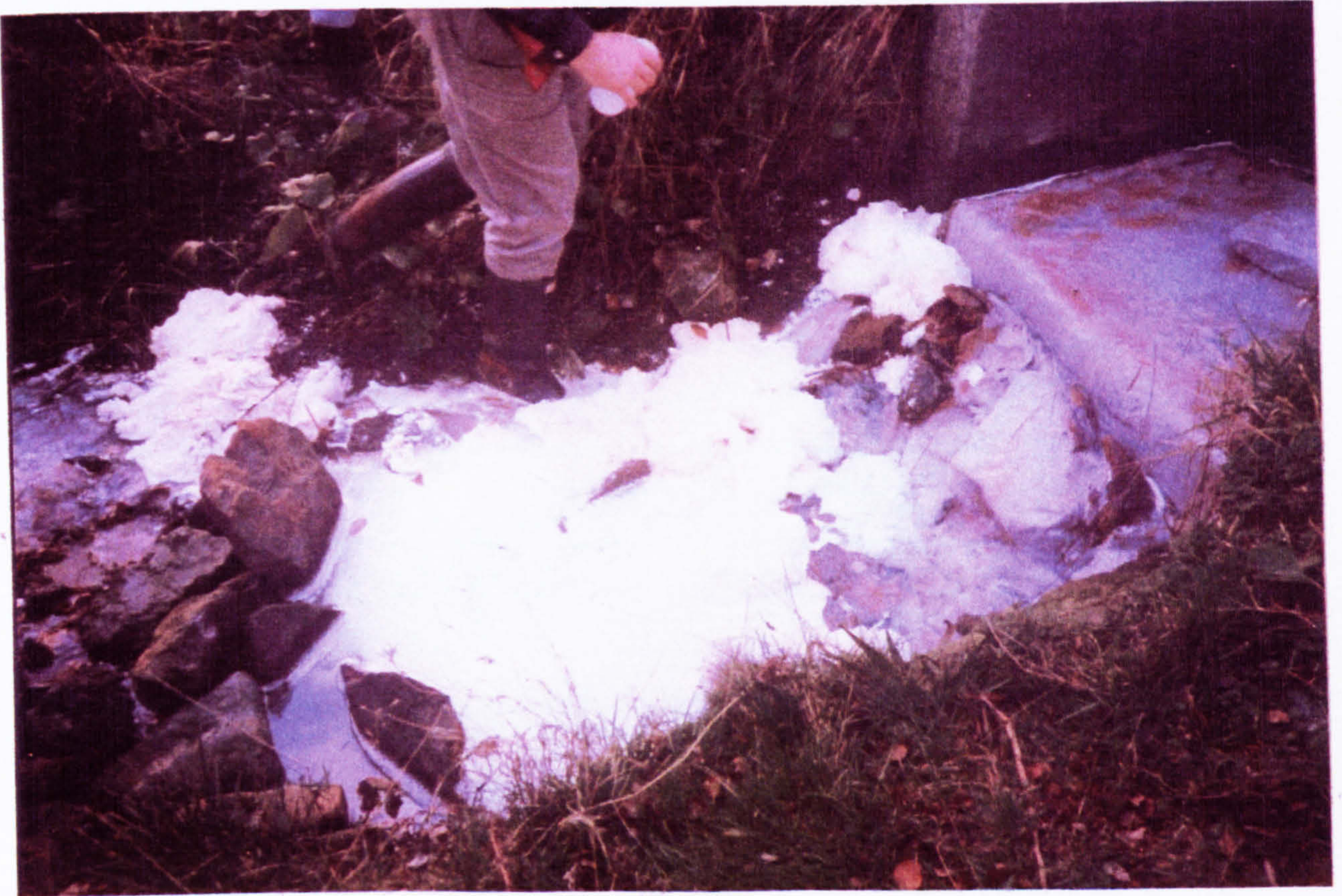
Figure 4.1 The Quaking Houses mine water discharging from a surface drainage system into the Stanley Burn in November 1994. The white discolouration of the streambed and unsightly 'froths' are aluminium hydroxide precipitates (photograph by Paul L. Younger, University of Newcastle upon Tyne).
