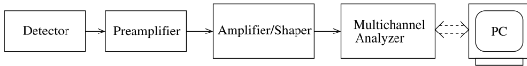
Figure 2.13: The signal processing of the detection system of alpha spectroscopy. [43]
