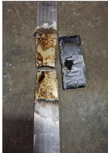
Figure 3. 18 Necking on the aluminium substrate after exposure at a constant heat flux of 112 kW/m 2 and 75 kN load
