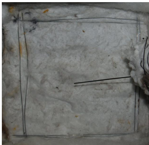
Figure 4. 9 No significant changes in kaowool sample after exposure to 116 kW/m 2 constant heat flux
