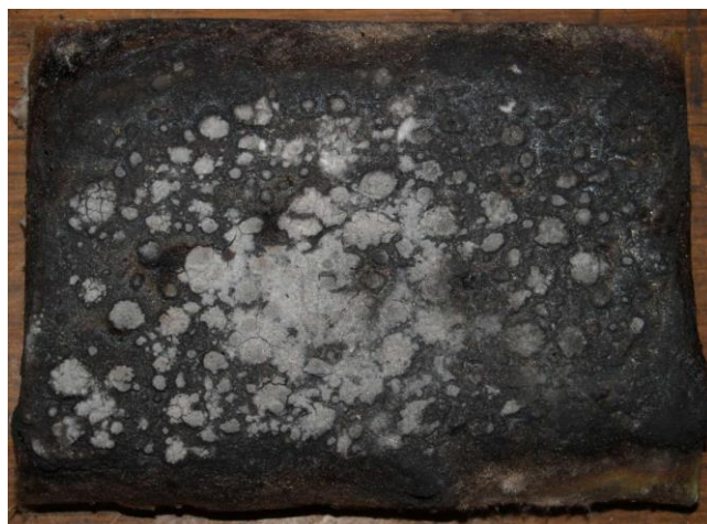
Figure 4.11 19 mm commercial intumescent coating after exposure to 116 \text{ kW/m}^2 constant heat flux
