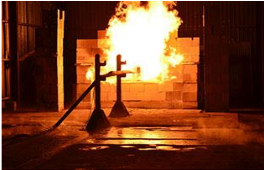
Figure 4. 1 Example of commercial jet fire testing in the oil and gas industries (Jotachar JF750)
