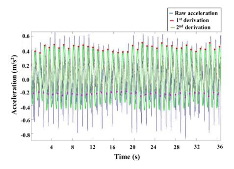
Figure 2: Raw Vertical Acceleration signal, 1<sup>st</sup> derivative, 2<sup>nd</sup> derivative, IC and FC event.
