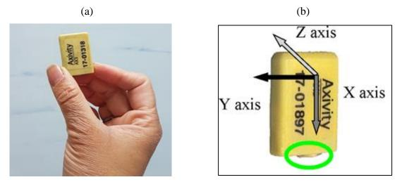
Figure 6-4: Body Worn Monitor (BWM) device
