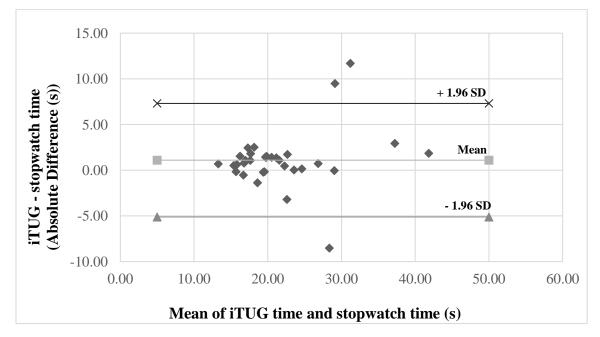
Figure 7-10: Bland-Altman Plot for Stopwatch TUG time vs iTUG time
