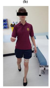
Figure 6-9: BWM on mid-thigh for community testing(a) Attachment of BWM on mid-thigh (port facing downwards) for measuring ambulatory PA(b) Participant walking with a BWM on mid-thigh
