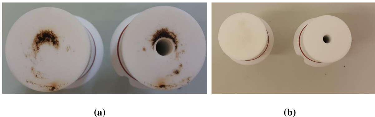
Figure 4.30. Photographs of the Macor caps in the NTP transmission cell (a) with and (b) without coating with \text{SnO}_2 nanopowder.
