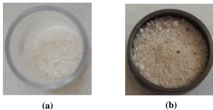
Figure 4.12. Photographs of the SnO 2 powder employed in the experiment in fig. 4.8 (a) before and (b) after the experiment.
