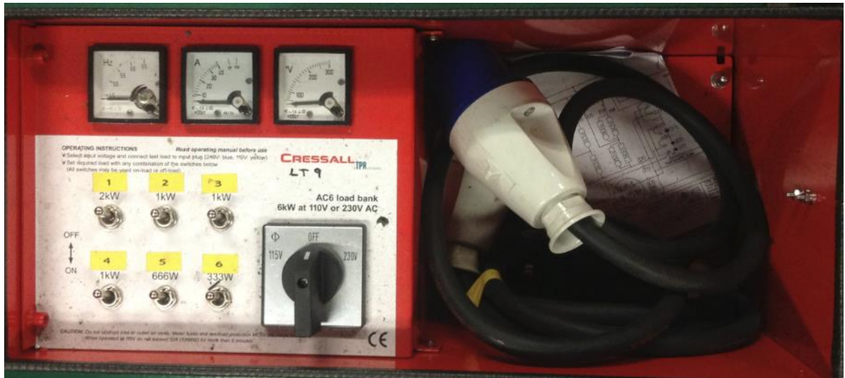
Figure 29 Load bank in the laboratory
