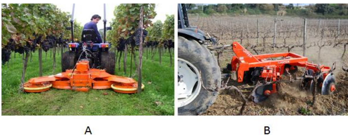
Figure 1.4 Mechanical weed control machines: A-in-row mower; B-Disc plough (Goldammer, 2013)
