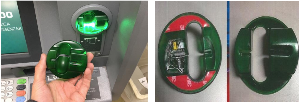
Figure 7 – Skimming devices found attached to ATM machines
