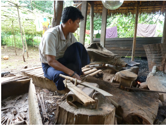
Picture 5.23: A blacksmith I interviewed in Dome village: he makes knives from recycled leaf-springs from trucks.
