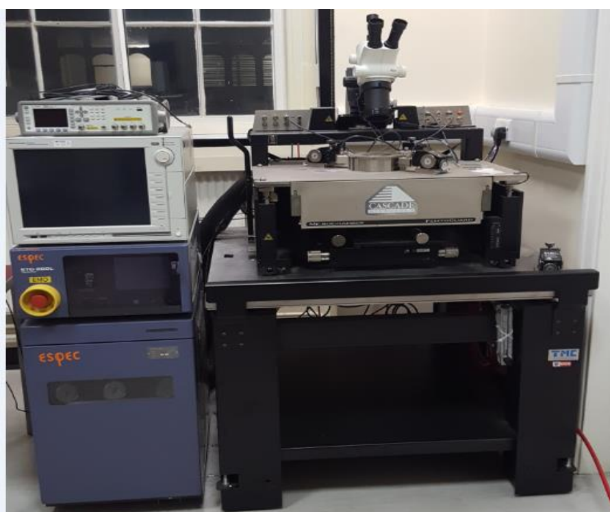
Figure 2.14 Photograph showing Hewlett Packard Agilent Technologies B1500A Semiconductor Device Analyzer attached with an ESPEC ETC-200L thermal chuck used for the I-V measurement at different temperature.
