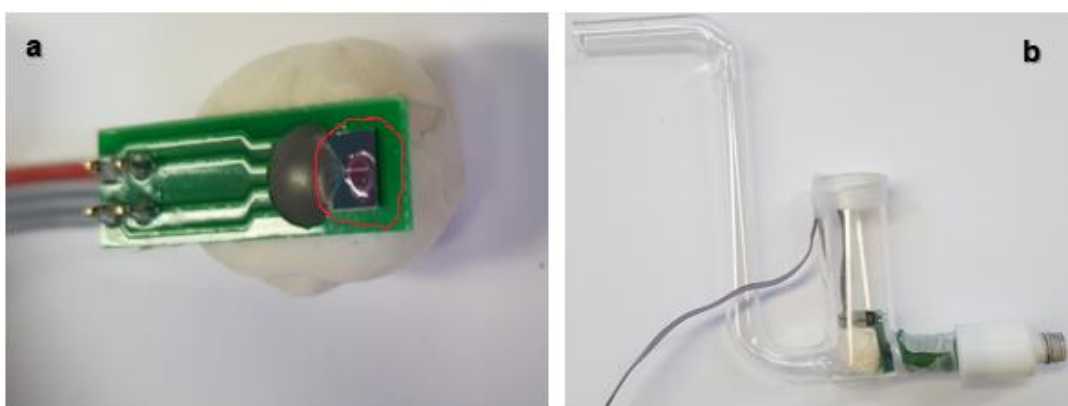
Figure 2.16 A photograph image of (a) the fabricated gas sensor showing the electrodes on which are aligned DNA templated nanowires (red circle) (b) the sensor device in a glass cell ready to be connected to the gas sensing set-up.
