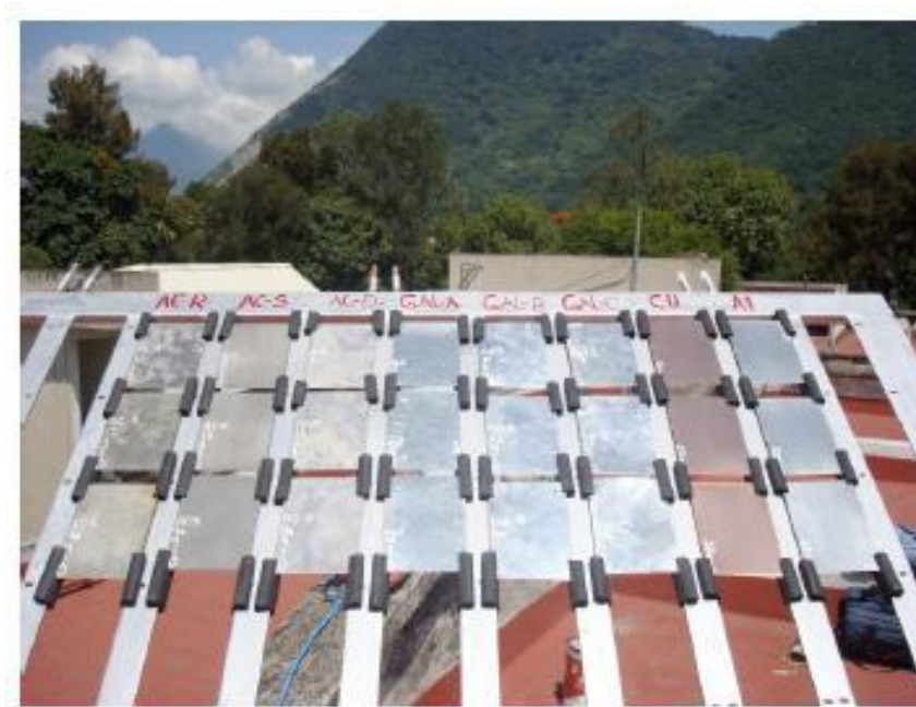
Figure 4. 3: Corrosion sample preparation in atmospheric environment
