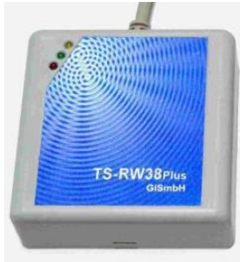
Figure 3.17: TS-RW38plus RFID reader kit from GiS-Net for programming tags
