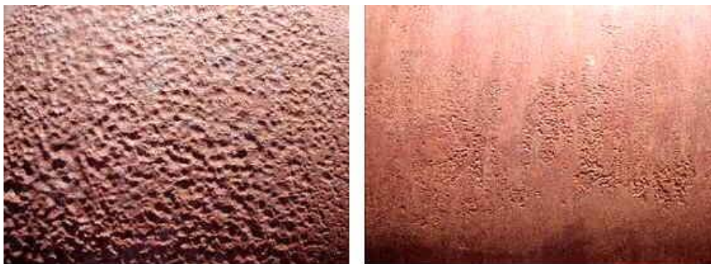
Figure 2.1: General corrosion patterns with major corrosion (left) to minor corrosion throughout the pipe surface (right) [20]
