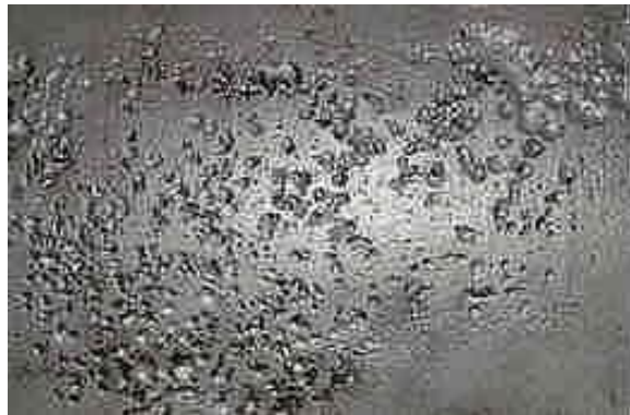
Figure 2.3: General pitting corrosion where smaller pits interconnecting to form larger pits [20]
