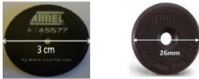
Figure 3.14: Commercially available off-the-shelf tags used in this study and their dimension
