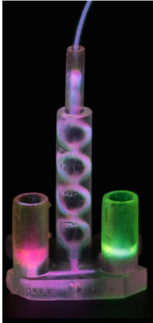
Figure 13. 3D micro-mixer with 1500 micron circular channel printed using Formlabs Form1+[146]
