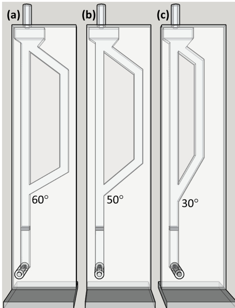
Figure 76. Schematic of the three system used to study the influence of the angle between the riser and solid feed pipe on the liquid-solid flow behaviour in a micro-circulating fluidised bed system. (a) With a 60^\circ angle between the riser and solid feed pipe, (b) with a 50^\circ angle between the riser and solid feed pipe, and (c) with a 30^\circ angle between the riser and solid feed pipe
