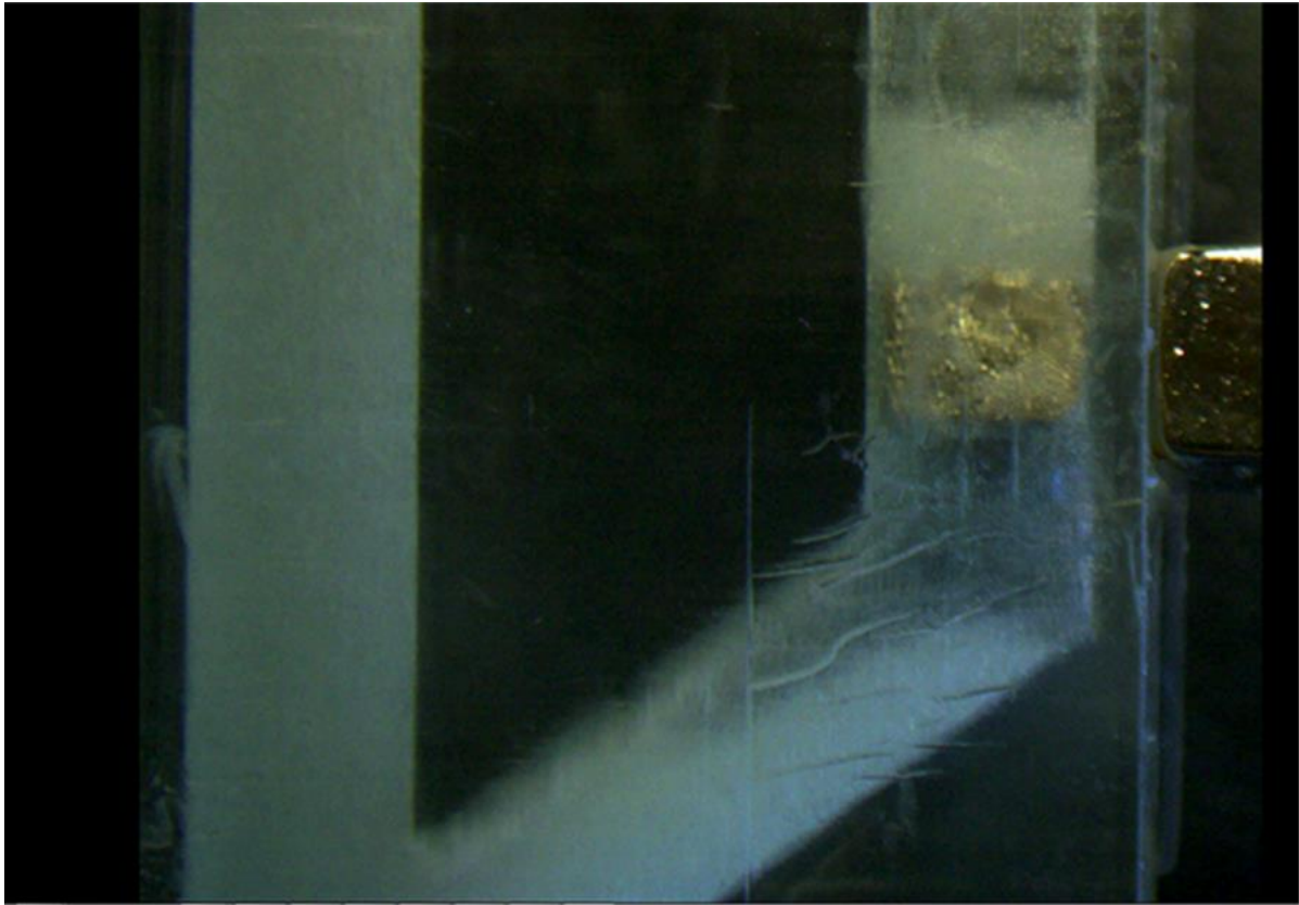
Figure 72. Picture of 3D printed micro-circulating fluidised bed with a magnet inside the system used to measure the solid circulation rate
