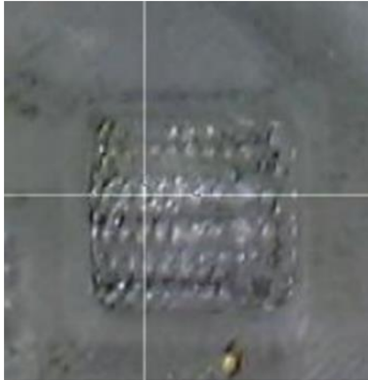
Figure 36. Printed cross-linked distributor of 150 \mu\text{m} diameter with 50 \mu\text{m} layer thickness
