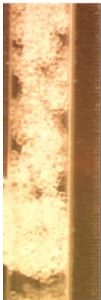
Figure 89. Optical Microscope illustrating agglomeration of 35 \mu\text{m} PMMA particle inside 1\text{mm}^2 micro-fluidised bed with water as the fluidising liquid.
