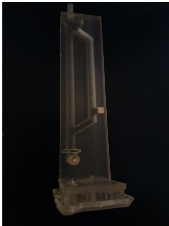
Figure 42. Displaying the 3D printed micro-circulating fluidised bed with a magnet inside the system used to measure the solid circulation rate
