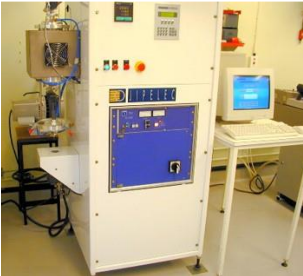
Figure 5-2: High temperature vacuum furnace (Newcastle University, School of Engineering).
