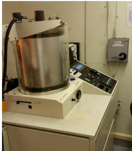
Figure 6-4: Edwards 306 e-beam evaporator in CLR4 (Newcastle University, school of Engineering).
