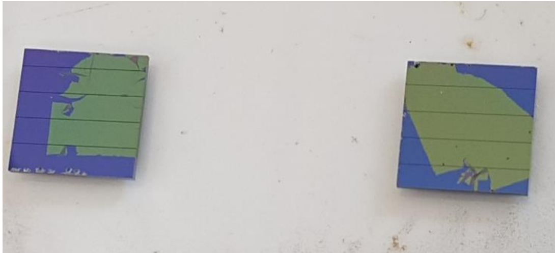
Figure 5-18: Graphene samples with sacrificial layer on the substrates after initial annealing process at 150 °C using hot plate.
