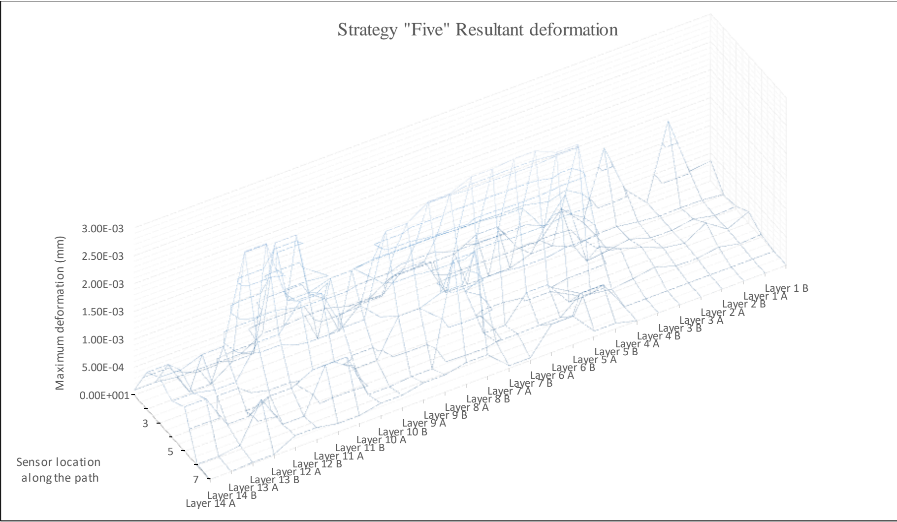
Figure 61: Maximum deflection recorded across of the thin wall structure using machining layer strategy “Five”
