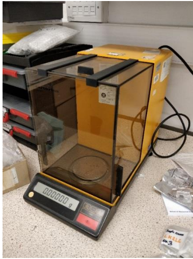
Figure 32: Sartorius Semi- Microbalance R 200 D
