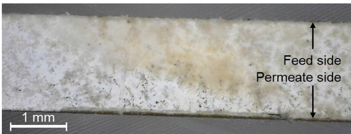
Fig. A. 16 Digital image of the cross-section of an Ag-sealed Al 2 O 3 -MC membrane after use. Feed-side inlet: 50 mol% CO 2 , 25 mol% O 2 in N 2 .
