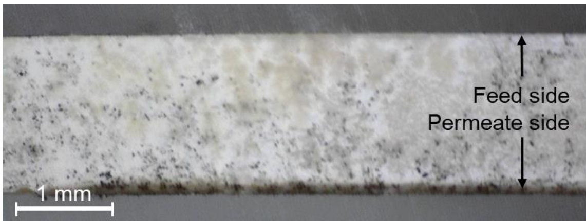
Fig. A. 15 Digital image of the cross-section of an Ag-sealed Ag/Al 2 O 3 -MC membrane after use. Feed-side inlet: 50 mol% CO 2 , 25 mol% O 2 in N 2 .
